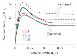
**Figure 7.3:** Nominal stress-strain tensile curves (up to  $\varepsilon_n=1$ ).
