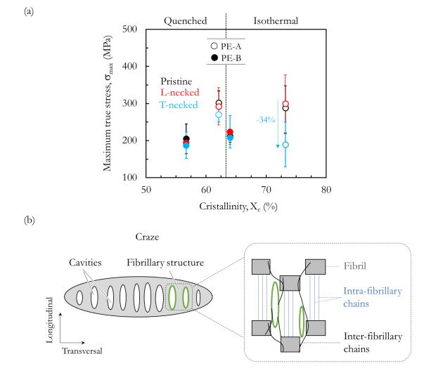
*Figure 11: a*) *Failure stress in different samples; b*) *schematic of craze and the heterogeneous ST distribution in the intra- and inter-fibrillary regions in PE-A isothermal sample who strongly cavitates.*
