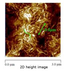
Figure 2.8: Observation of percolated crystalline structure by AFM[18].
