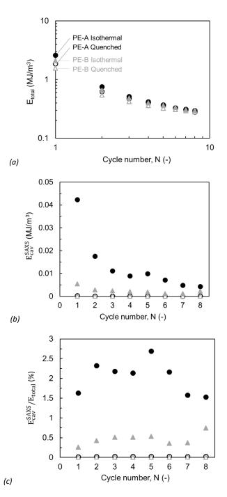
**Figure 9:** Energy profiles plotted as a function of the cycle number: (a) Total dissipated energy per unit volume Etotal; (b) dissipated energy per unit volume due to cavitation  $E_{cav}^{SAXS}$ ; (c)  $E_{cav}^{SAXS}$  / Etotal ratio as a function of cycle number.
