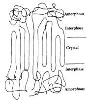
Figure 2.5: Amorphous-interphase-crystalline structure[20].
