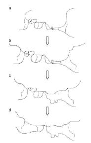
Figure 5.13: Microstructure evolution associated with stress softening[104]
