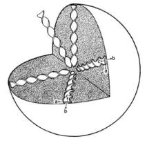
Figure 2.9: Schematic of spherulitic structure[8].
