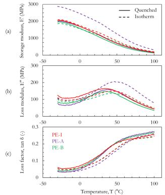
Figure 8.3: Evolution of visco-elastic properties as a function of temperature.
