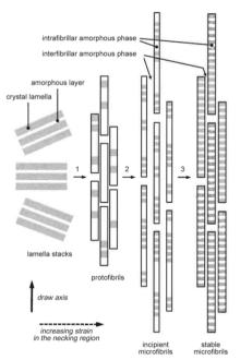
Figure 5.4: schematic of fibrillar transformation[75].
