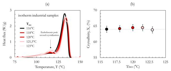
**Figure 5.4:** (a) DSC curves for the isotherm industrial samples with different  $T_{iso}$  in the vicinity of the melting temperature (endo up); (b) crystallinity of isotherm samples as a function of treating temperature  $T_{iso}$ .
