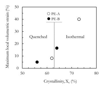
*Figure 4:* Maximum local volumetric strain at the final zero-stress state as a function of sample crystallinity
