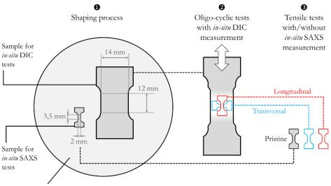
PE sheet shaped with different thermal treatments
