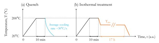
*Figure 4.3:* Temperature profiles of the quenching and isothermal treatments: (a) quench; (b) isothermal treatment.
