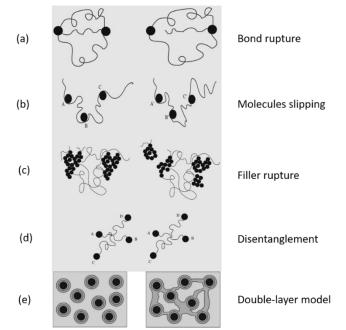
*Figure 5.11:* Physical mechanisms to interpret the Mullins effect in filled rubbers: a) bond rupture; b)molecules slipping; c) filler rupture; d) disentanglement; e) double-layer model [100]
