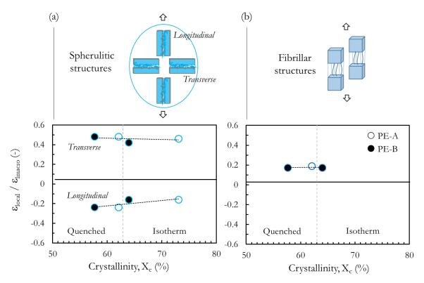
Figure 9: local/macro strain ratios in pristine and pre-loaded samples<sup>16</sup>.
