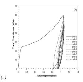
*Figure 4.2: a*) Stress-controlled cyclic loading mode[53]; b) Strain-controlled cyclic loading mode[54]; c) Mixed cyclic loading mode[59]
