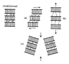
Figure 5.2: a) Inter-lamellar shear; b) inter-lamellar separation; c) stack rotation[66]
