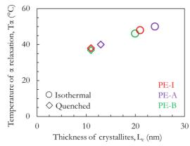
Figure 8.4: Temperature of a relaxation as a function of thickness of crystallites.
