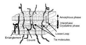
Figure 2.6: Stress transmitters in semi-crystalline polymers.
