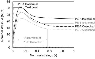
Figure 1: Tensile curves and measurement of neck width.
