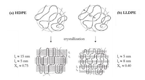
Figure 2.7: Schematic of formation of tie molecules during crystallization (adapted from[21]).
