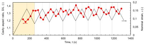
*Figure 13:* Time evolution of the cavity aspect ratio and applied nominal strain in the PE-B Isothermal sample under mixed-mode oligo-cyclic test.
