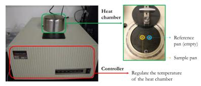
Figure 5.2: Perkin-Elmer DSC7 apparatus.
