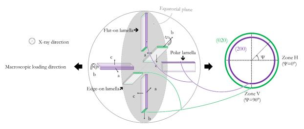
*Figure 3:* Location of equatorial and polar lamellae in spherulite and identification of the WAXS scattering patterns.
