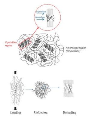
Figure 5.14: Network alteration during loading-unloading-reloading[58].
