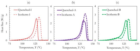
*Figure 5.5:* DSC curves of the quenched and isotherm samples in the vicinity of the melting temperature (endo up): (a) PE-industrial; (b) PE-A; (c) PE-B.
