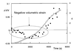
Figure 5.3: Volumetric and true axial strains, as a function of drawing time at 20°C [69].
