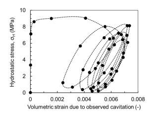
*Figure 8:* Hydrostatic stress as a function of the volumetric deformation due to observed cavities in PE-A Isothermal sample.
