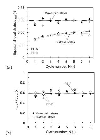
**Figure 4:** (a) Local strain at maximum-strain and minimum-stress states. (b) Plot of ratio  $\varepsilon_{local}/$  $\varepsilon_{macro}$  as a function of cycle number (quenched samples).
