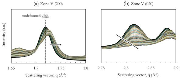
*Figure 4*: Shift of WAXS peaks in Zone V under macroscopic tension (a) (200) peak; (b) (020) peak.
