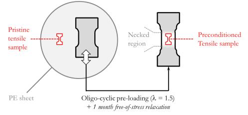
Figure 1: Pristine and pre-loaded sample preparations
