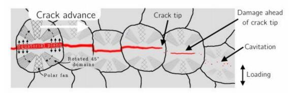
Figure 5.6: Fatigue damage progression by intra-spherulitic failure in the equatorial plane[85]
