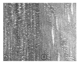
Figure 5.5: Cavitation between lamellae and longitudinal coalescence[84].
