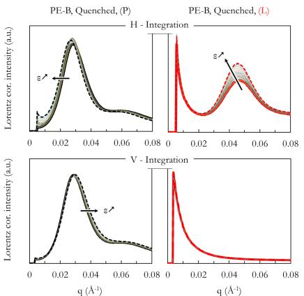
**Figure 7:** Lorentz-corrected intensities (Iq<sup>2</sup>) as a function of the norm of the scattering vector q in horizontal (H) and vertical (V) regions of the SAXS pattern for the Pristine (P) and L- necked (L) samples of the PE-B quenched material.
