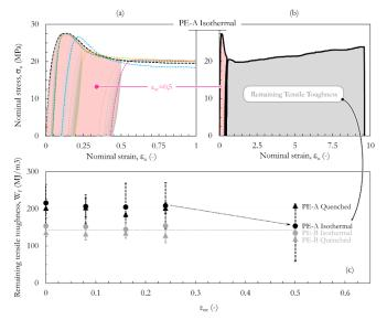
$\label{eq:Figure 12: a) Mullins-like behavior of PE-A isothermal sample; b) Definition of remaining tensile toughness (ex. PE A isothermal sample, with $\epsilon_{OC}=0.5$), c) Remaining tensile toughness in different samples as function $\epsilon_{OC}$$
