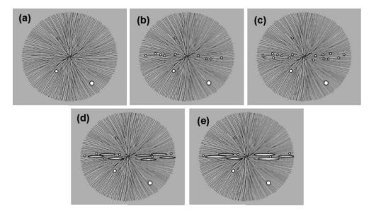
*Figure 5.8:* Growth of submicrometer cavities in the amorphous phase between lamellae oriented in the direction normal to the applied stress. (a) Micrometer-sized cavities with broad distribution of size in the nonfatigued sample. (b) Nucleation of cavities in the amorphous phase with diameters comprised between 20 and 180 nm. (c) Increase of the number of the spherical cavities in the course of fatigue testing. (d, e) Growth of the cavities in the direction normal to the applied stress[38].
