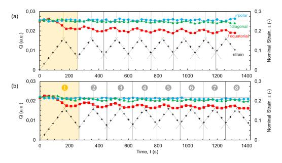
**Figure 5:** Evolution of Q value at different region of spherulite/applied macro-strain as a function of time: (a) PE-A Quenched sample; (b) PE-B Quenched sample.
