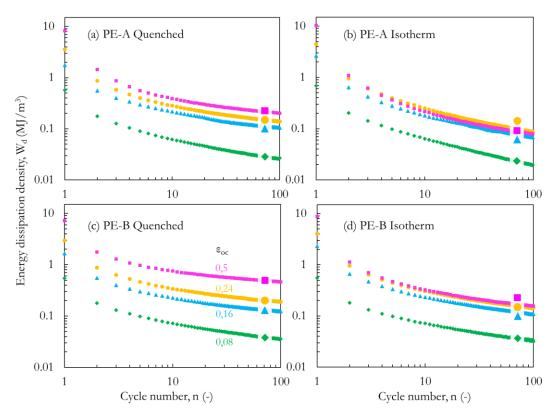
**Figure 7:** Density of energy dissipation  $W_d$  as a function of cycle number in PE samples with different applied oligo-cyclic strains  $\varepsilon_{OC}$ : (a) PE-A Quenched; (b) PE-A Isothermal; (c) PE-B Quenched and (d) PE-B Isothermal
