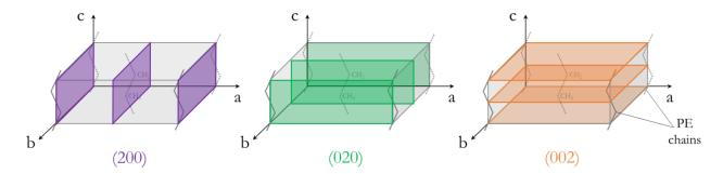
**Figure 2:** Illustration of prescribed planes in a PE crystal orthorhombic cell related to crystallographic strains along *a*, *b* and *c* axes.
