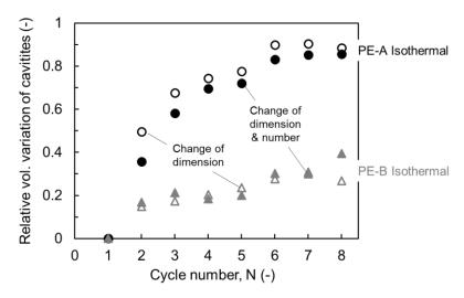
*Figure 12:* Variation of unit/total cavity volume at zero stress states as a function of the cycle number.
