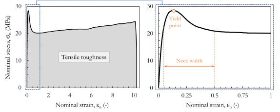
Figure 7.1: Nominal stress-strain curves and some important mechanical indictors.
