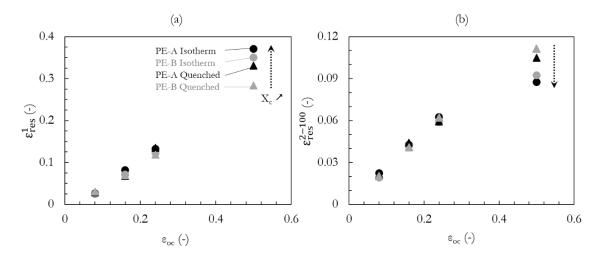
Figure 6: Change of the residual strains as a function of the prescribed maximum strain a) after the 1<sup>st</sup> cycle, b) from 2<sup>nd</sup> to 100<sup>th</sup> cycle
