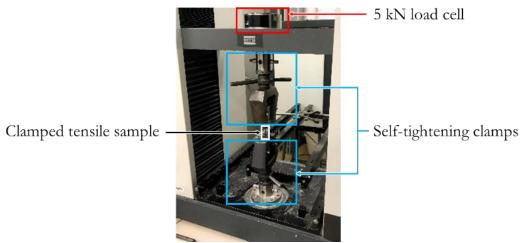
Figure 7.2: MTS 1/ME machine equipped with 5kN load cell.
