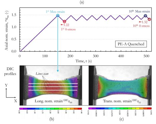
**Figure 2:** Results of in-situ DIC measurement of PE-A quenched sample: (a) strain loading profile prescribed by the testing machine; (b) longitudinal strain mapping at the end of the first loading; (c) transversal strain mapping at the end of the first loading.
