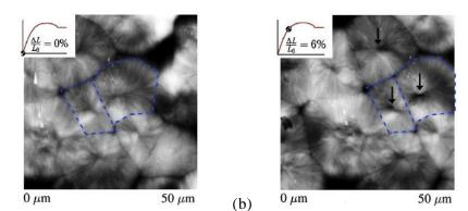
*Figure 5.10: AFM observation of fragmentation of lamellae in the pre-yield regime*[92]
