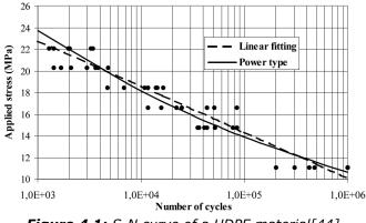
Figure 4.1: S-N curve of a HDPE material[44]
