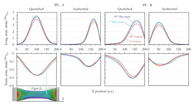
**Figure 3**: Longitudinal (L.) and transversal (T.) nominal strain distributions as a function of Xposition at 4 stages during the oligo-cyclic test (N.B. the bottom left image recalls the transverse nominal strain field at the end of the first loading step).
