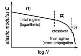
Figure 5.9: Schematics of the modulus evolution with increasing cycles during fatigue tests[38].
