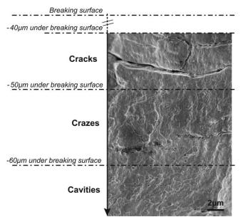
*Figure 5.7:* Cryofracture in the direction parallel to the stress in neat PA after fatigue failure (SEM) [38].
