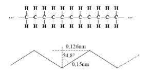
*Figure 2.1:* Molecular structure of a PE long chain[8] (N.B. the bottom figure details the geometrical peculiarity of the C-C-C bond).
