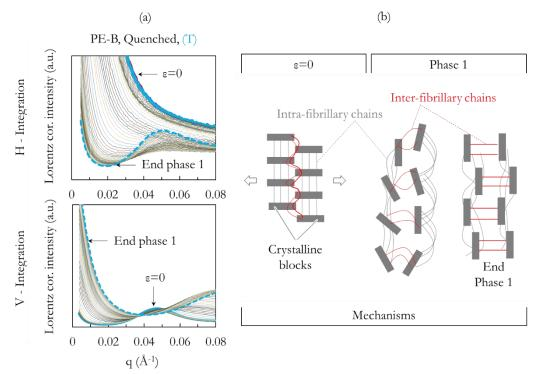
**Figure 10:** a) Lorentz-corrected intensities (Iq<sup>2</sup>) as a function of the norm of the scattering vector q at horizontal and vertical zones of the SAXS pattern for the T-necked PE-B quenched sample; b) Schematic of the reorientation of crystalline blocks during the tensile deformation of T-necked samples.
