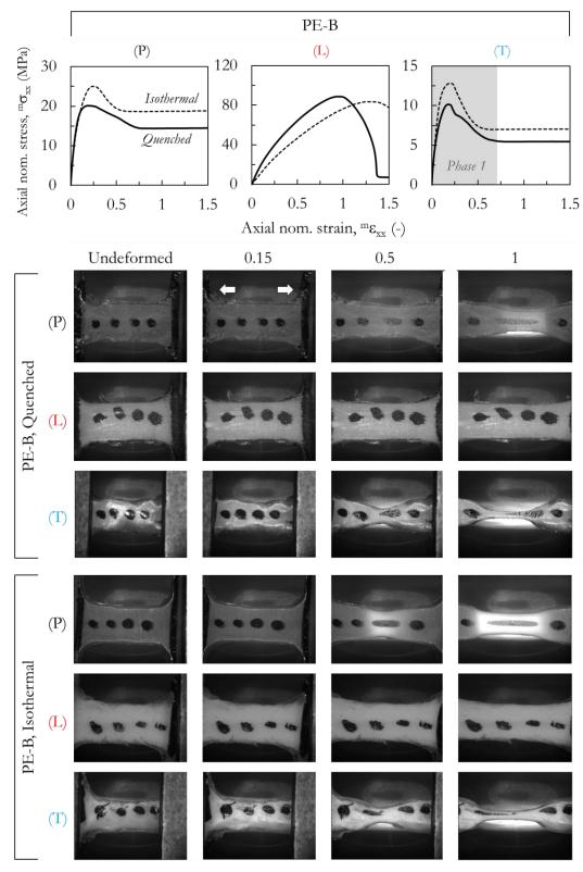
*Figure 5:* Tensile nom. stress - nom. strain profiles in the pristine (P), L-necked (L) and T-necked (T) samples of PE-B materials (on top). Companion pictures of the specimen for four stages (on bottom).
