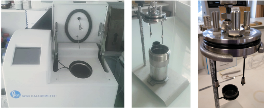
Figure 52. Calorimeter employed for the determination of the combustibility of the samples: a) The whole machine with the screen for the results and oval vessel with water in which the calorimetry pump is introduced, b) Calorimetry pump with pressurized sealing and releasing valves, c) Pan for the sample in contact with the wire, which created the spark for the combustion.
