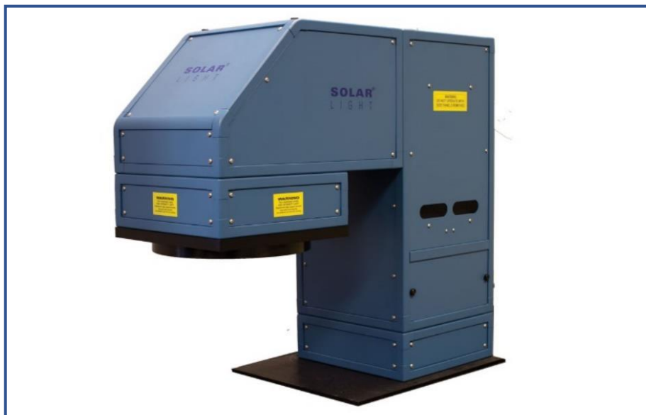
Figure 28. LS1000 Solar Simulator used by our laboratory, CIBEST/CEA . The photo was taken from the original website for purchasing this model. (“6" (15.25 Cm) 1000W PV Cell Testing Solar Simulator Kit Model LS1000-6R-002 - Solarlight” n.d.).
