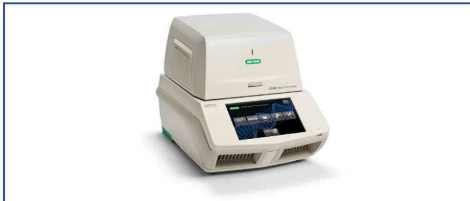
Figure 30. The CFX96 thermal cycler C1000-touch used by our laboratory, CIBEST/CEA. It monitors the amplification of targeted short DNA fragments in real-time.
