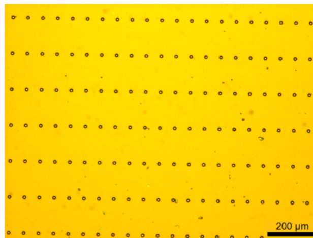
Figure 7.6 Top view optical microscope image of PEALD insulated sample after the insulation validation.
