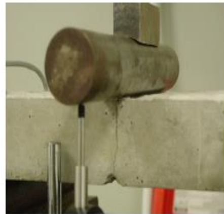
(b) Closing of crack after healing
