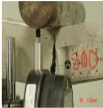
(a) Crack formation during loading
