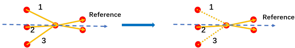
Figure 7.4: The illustration of how to clean the connectors of a hit in the Arbor PFA. The blue dashed arrows are reference direction and the orange dotted lines represent the connectors removed.
