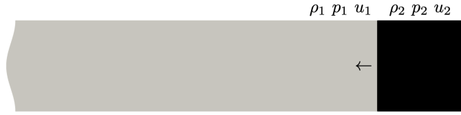
Figure 7.2: Geometrical set-up and initial conditions for shock/wavy-wall interaction.
