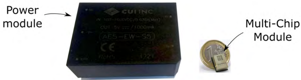
Figure 6: Example of size comparison of a power module [2] and a Multi-Chip Module [1]
