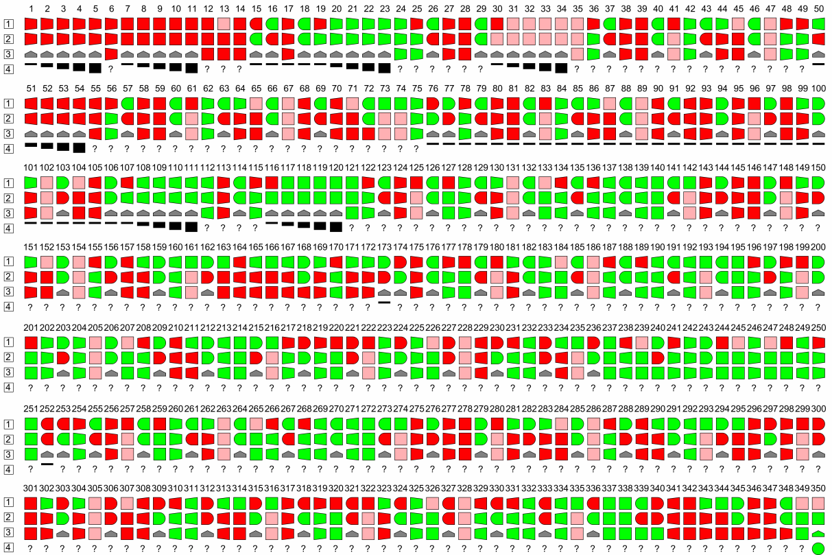
Figure 5.8: Trace of the first 350 interaction cycles in our experiment. Line 1: intended interactions. Line 2: enacted interactions. Line 3: belief states: unknown (grey triangle) / known state represented by its corresponding persistent interaction. Line 4: mood: curious (question mark), excited (increasing black bars), or confident (green circle).
