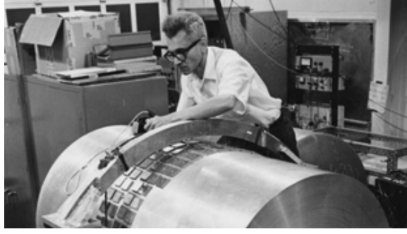
Fig. 1.15 Joseph Weber and its aluminium bar detector.
