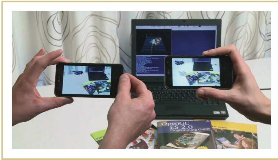
Figure 2.3 – By sharing components, multiple devices can track and expand the same map and recognize the same objects [1].
