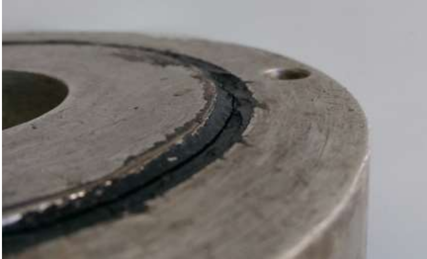
Figure 5-17 Bottom part of Bm_ASR_sp2 sample after LRP test at high loading amplitude (10800 \mu\text{m}/\text{m} )
