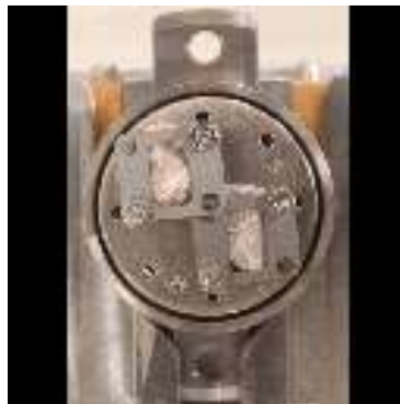
Figure 3-14 Two road aggregates ( D \approx 1\text{cm} ) clamped onto the XPS testing plate
