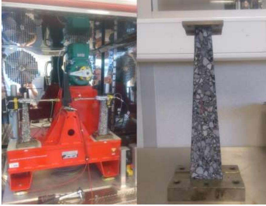
Figure 3-7 Vectra® 2PB apparatus and trapezoidal mixture specimen (height = 250mm), courtesy of Eiffage Company
