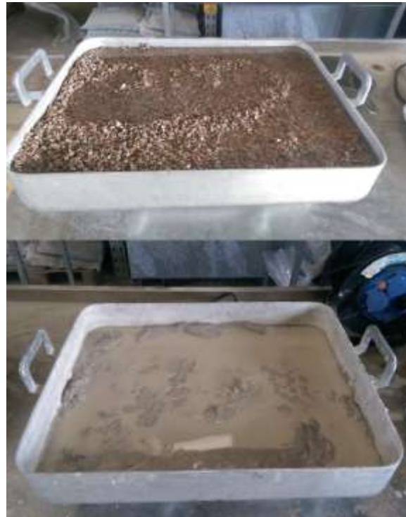
Figure 7-2 Trays of CO aggregates and HL filler during the evaporation phase of the silanisation procedure
