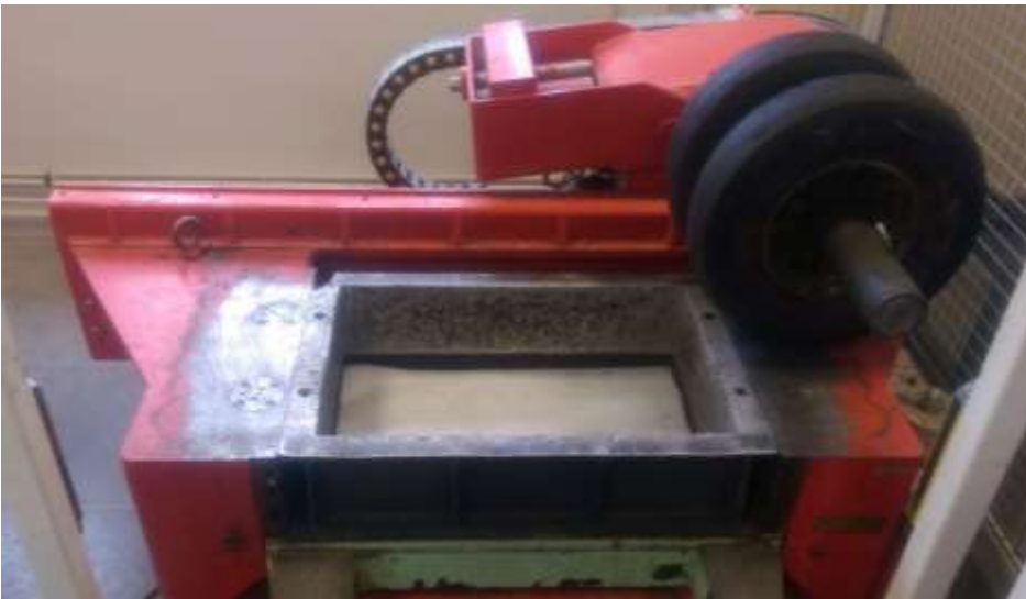
Figure 3-9 Roller compactor, courtesy of Eiffage Company
