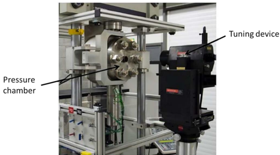
Figure 1.26 Optical tracking experimental set up (Kane Diallo 2016)
