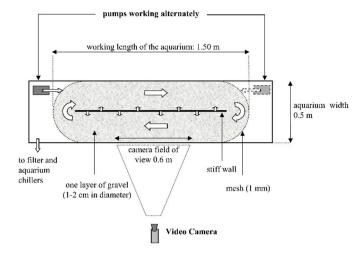
Fig. 2. Diagrammatic top view of the annular flume.
