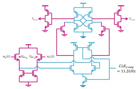
Figure 5-29: Clocked comparator's topology
