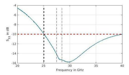
Figure 5-40: S<sub>11</sub> parameter characterizing the input matching of the SDM
