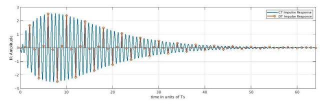
Figure 4-28: Continuous and Discrete Time Feedback Impulse Response over 64 sampling periodes
