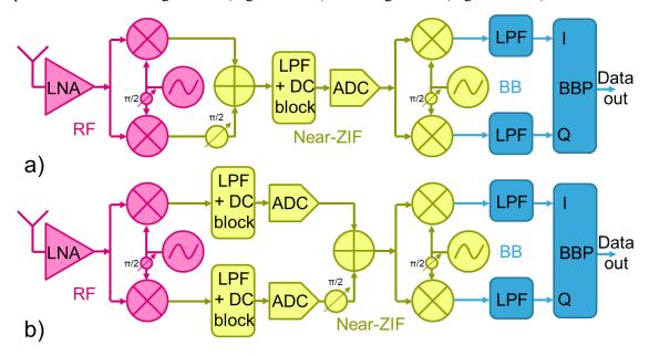
Figure 3-14: Near-ZIF receiver using the Hartley image cancelling approach a) with an analog implementation, b) with a digital implementation
