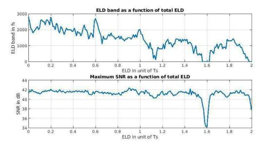
Figure 4-47: Top) ELD band for modulators with per design ELD between  $0 \times T_S$  and  $2 \times T_S$ .
