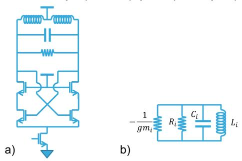
Figure 5-23: a) Negative-gm circuit topology. b) Principle single ended equivalent.
