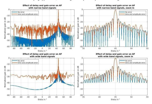
Figure 2-20: Top graphs: Impact of delay and gain error on Array Factor for narrow band signals
