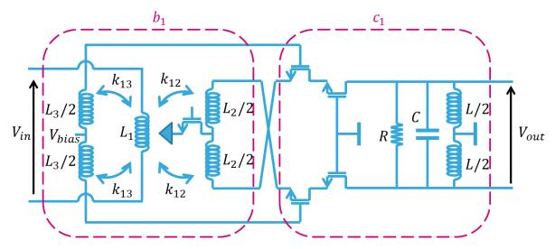
Figure 5-4: gm-boosted common gate LNA with tranformer feed
