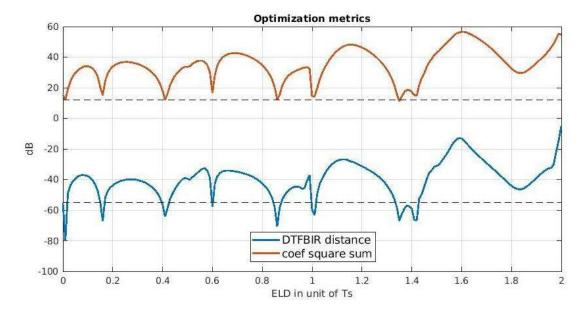
Figure 4-44: DTFBIR distance to reference modulator and feedback coefficients' square sum versus ELD
