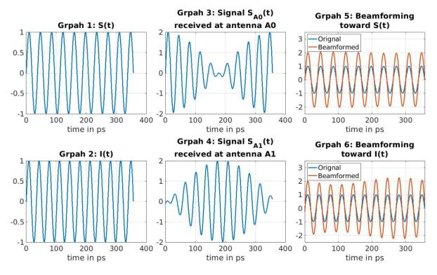
Figure 2-4: Plots of incoming plane waves, antenna received signals and beamformed signals
