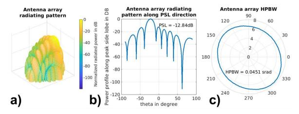
Figure 2-10: 64 element UPA a) Radiation Pattern b) Profile along PSL c) HPBW contour
