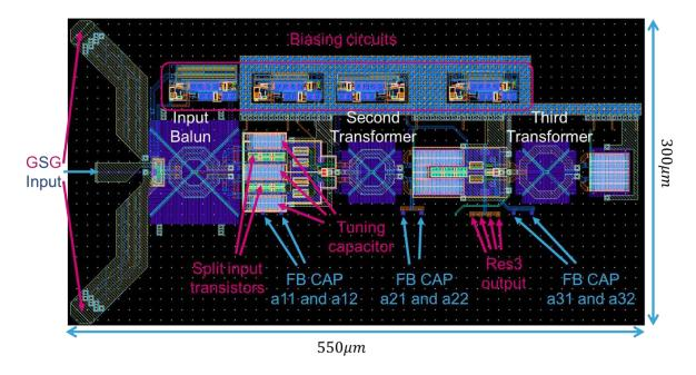
Figure 5-39: Feed forward analog path layout
