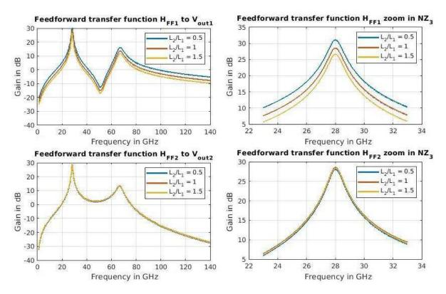
Figure 5-18: Feedforward transfer functions variations when sweeping the ratio  $L_2/L_1$
