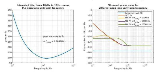
Figure A.3.3: Left) Integrated jitter from 10 kHz to 1 GHz versus PLL open loop unity gain frequency. Right) PLL output phase noise for different open loop unity gain frequency
