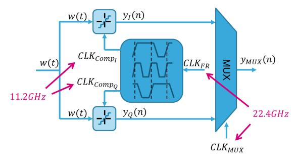
Figure 5-24: Time-interleaved quantizer principle schematic
