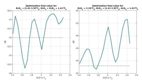
Figure 4-49: ELD<sub>1</sub> and ELD<sub>2</sub> scan for optimization's first step
