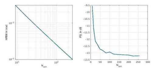
Figure 2-11: HPBW (left) and PSL (right) for square UPAs versus the number of antennas Nant.
