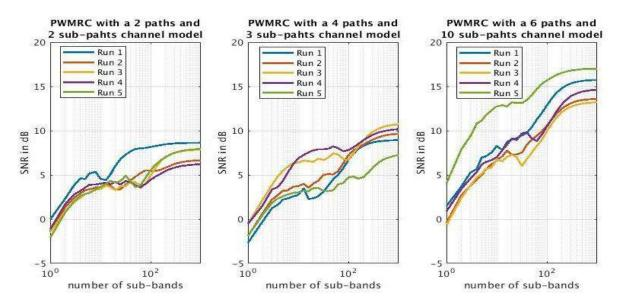
Figure A.2.2: SNR vs the number of sub-bands under MRC beamforming from 3 different channels
