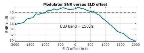
Figure 4-50: ELD robustness test on a modulator with individually optimized
