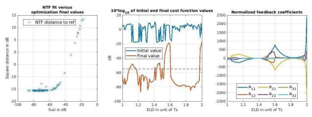
Figure 4-39: Optimization results for ELD values from 1 to 2  $T_S$  using the refined procedure
