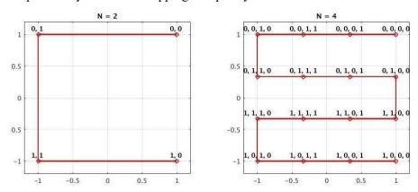
Figure 3-6: Symbol mapping for 2-bit symbols on the left and 4-bit symbols on the right
