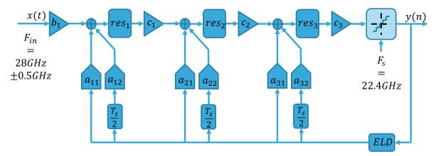
Figure 5-1: Modulators architecture
