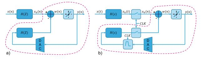
Figure 4-13: Alternate representation of a) Discrete time sigma-delta modulators b) Continuous time sigma-delta modulators
