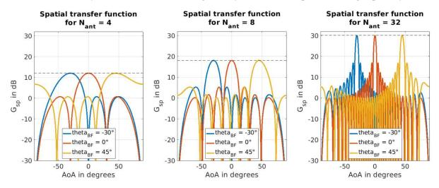
Figure 2-6: Spatial transfer function for ULAs with 4, 8 and 32 antennas for various beamforming angles
