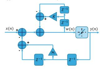
Figure 4-8: Simulation model of a second order BPDTSDM
