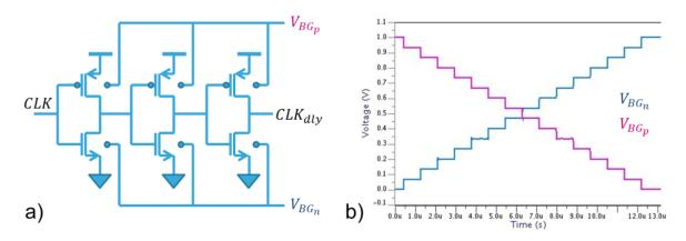
Figure 5-35: a) Tunable delay cell topology. b) Static control DAC characteristic.
