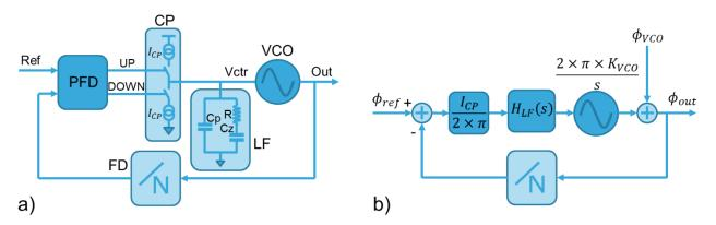
Figure 3-4: a) PLL Classical implementation b) Equivalent Linear Time Invariant (LTI) model
