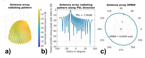
Figure 2-12: 64 element UCA a) Radiation Pattern b) Profile along PSL c) HPBW contour
