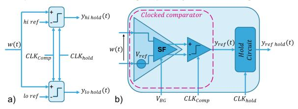
Figure 5-28: Quantizer and latching comparator principle schematics
