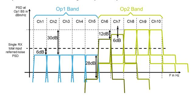
Figure 2-30: Op1 S-BS single receiver PSD profile
