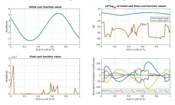
Figure 4-33: Optimization results for ELD values from 0 to  $T_S$
