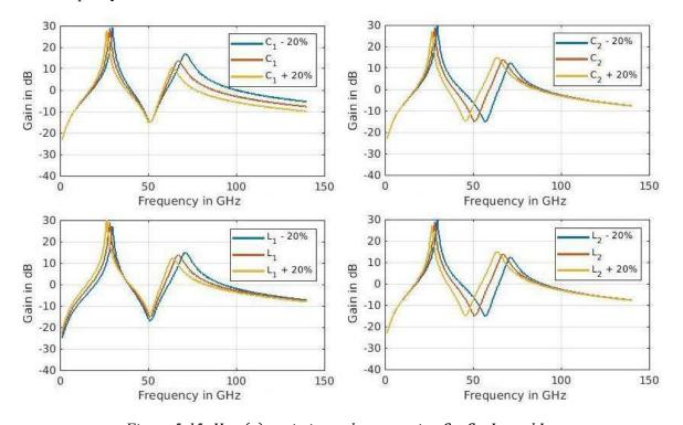
Figure 5-15:  $H_{FF_1}(s)$  variations when sweeping  $C_1$ ,  $C_2$ ,  $L_1$  and  $L_2$ .
