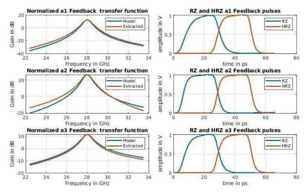
Figure 5-42: Left graphs, from top to bottom: First, second and third feedback transfer functions. Right graphs, from top to bottom: First, second and third feedback pulses for the RZ and HRZ DACs.
