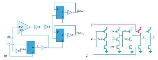
Figure 5-25: a) I and Q half rate clock generator b) True Single Phase Clock D-flip-flop topology
