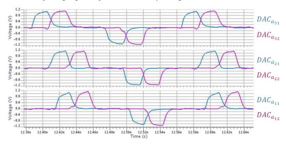
Figure 5-37: Feedback DACs' differential outputs
