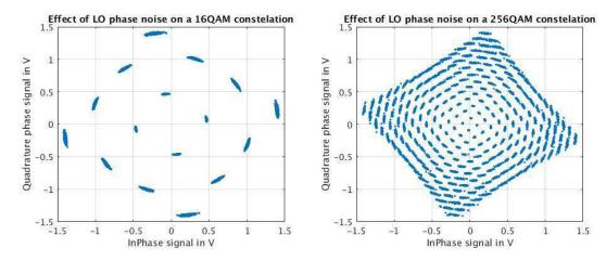
Figure 3-8: Impact of phase noise on received QAM symbols for 100us long symbol stream at 100Msymbols/s
