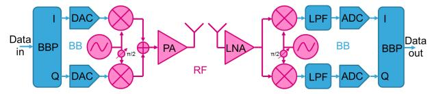
Figure 3-7: Block diagram of a wireless transmission chain with homodyne transmitter and receiver
