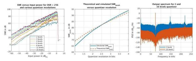
Figure 4-10: Simulation of a second order BPDTSDM for various quantizer resolution. Left: SNR versus input power. Middle: Theoretical and simulated peak SNR. Right: Output spectrum for a 2 and a 16 level quantizer
