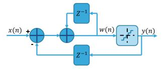
Figure 4-5: Simulation model of a first order LPDTSDM
