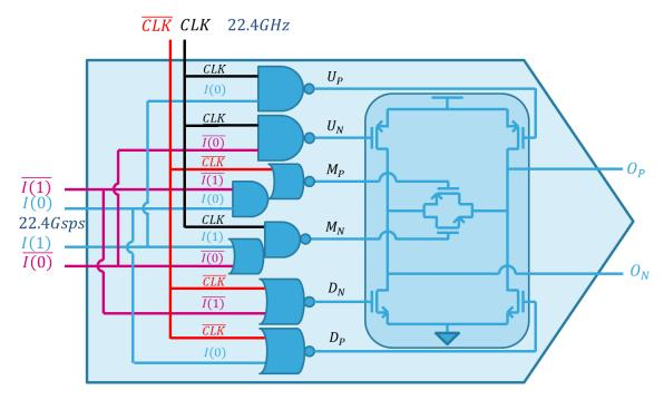
Figure 5-9: Feedback RZ Voltage DAC topology
