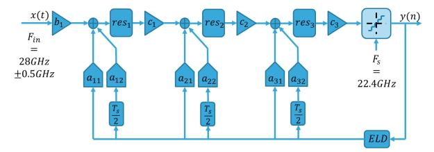
Figure 5-1: Modulators architecture
