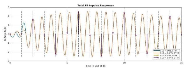
Figure 4-32: Comparison of modulators' feedback impulse responses for 0 and  $0.4 \times T_S$  ELD modulators
