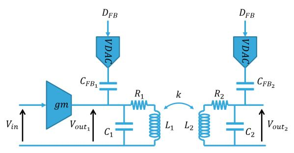
Figure 5-13: Proposed Transformer based gm-LC resonator
