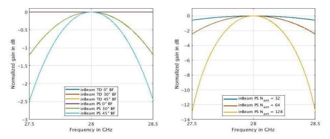
Figure 2-17: In Beam frequency response of time delay versus phase shift beamforming. Left: ULA with 64 elements for steering angles of 0°, 30° and 45°. Right: Steering angle of 45° using phase shift beamforming for ULAs with 32, 64 and 128 elements
