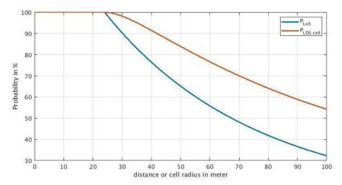
Figure 2-25: LoS probability for a user at distance d and average LoS probability in a cell of radius r
