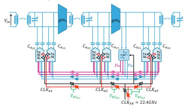
Figure 5-34: Modulator's simplified implementation schematic
