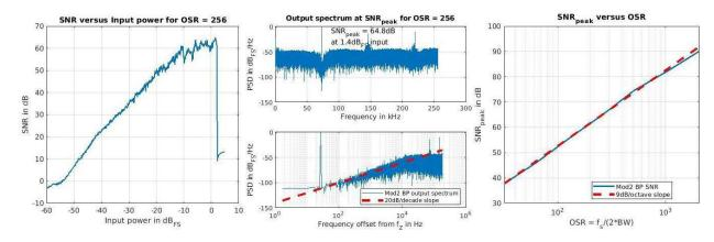
Figure 4-9: Simulation of a second order BPDTSDM. Left: SNR versus input power. Middle: Output spectrum at SNR<sub>peak</sub>. Right: SNR<sub>peak</sub> versus OSR
