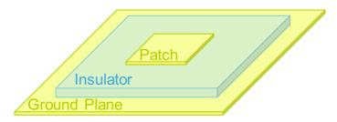
Figure 2-16: Basic architecture of a patch antenna
