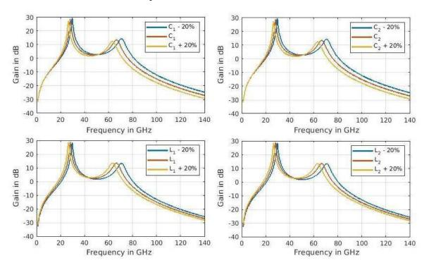
Figure 5-16:  $H_{FF_2}(s)$  variations when sweeping  $C_1$ ,  $C_2$ ,  $L_1$  and  $L_2$ .  $\sim 171 \sim$
