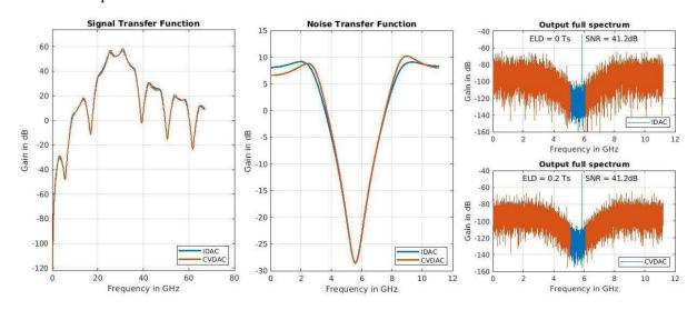
Figure 5-7: Comparison between an IDAC and CVDAC modulator
