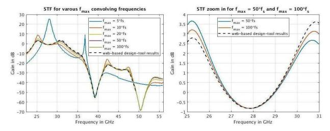
Figure 4-27: STF versus maximum convolving frequency
