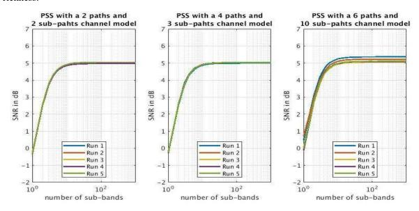
Figure A.2.1: SNR vs the number of sub-bands under PSS beamforming from 3 different channels
