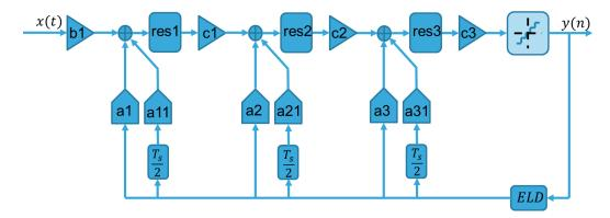
Figure 4-25: Modulator's architecture
