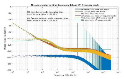
Figure 3-5: Phase Noise of a matlab time domain implementation of the PLL versus the LTI frequency model with a center frequency of 22.4GHz
