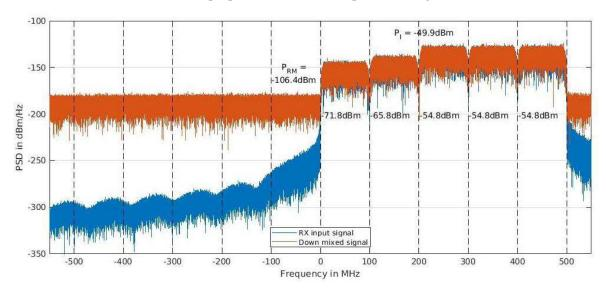
Figure 3-11: Evaluation of reciprocal mixing between a modulated interferer and a noisy LO
