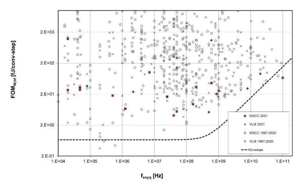
Figure 3-16: Walden Figure of Merit versus sampling frequency
