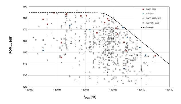
Figure 3-17: Schreier Figure of Merit versus sampling frequency
