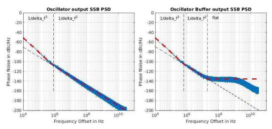
Figure 3-3: Typical Single Side Band PSD of a free running oscillator on the left and of its limiting amplifier output on the right
