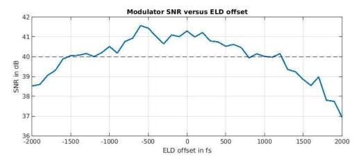
Figure 4-46: Reference modulator SNR versus ELD offset from -2ps to 2ps with a step of 100fs
