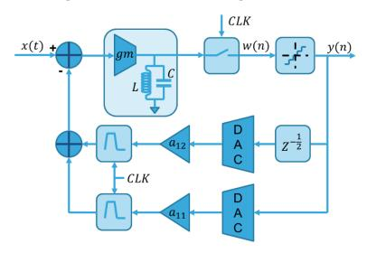
Figure 4-16: BPCTSDM parametric architecture
