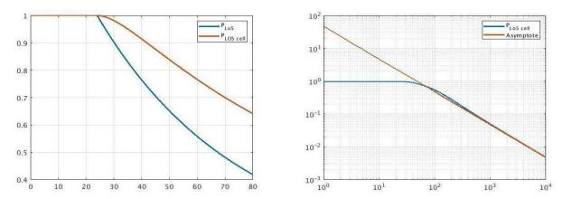
Figure A.2.3: Left  $P_{LoS}(d)$  and  $P_{LoS_{Cell}}(d_{SC})$ . Right)  $P_{LoS_{Cell}}(d_{SC})$  and its asymptote at infinity on a log-log plot
