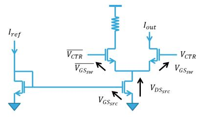
Figure 5-5: Simple implementation of a current steering DAC
