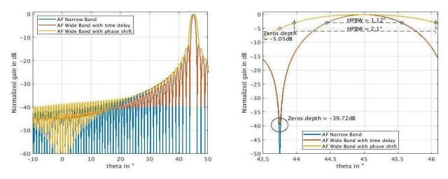
Figure 2-18: Array factor for a 128-element ULA for narrow and wide band signal with time delay and phase shift beamforming
