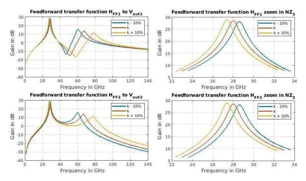
Figure 5-17: Feedforward transfer functions variations when sweeping k
