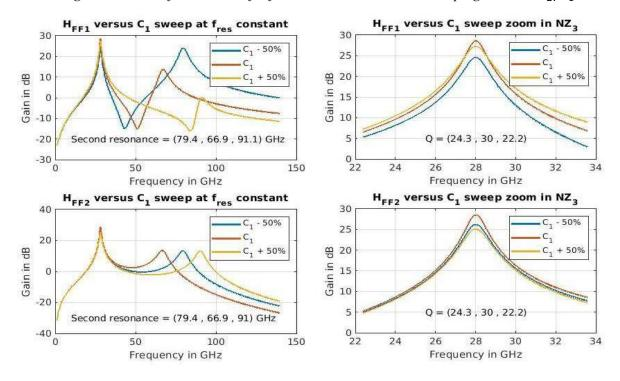
Figure 5-19: Feedforward transfer functions variations when sweeping  $C_1$ , with  $L_1 = L_2 = 400 pH$  and adjusting  $C_2$  for a constant 28GHz resonating frequency.
