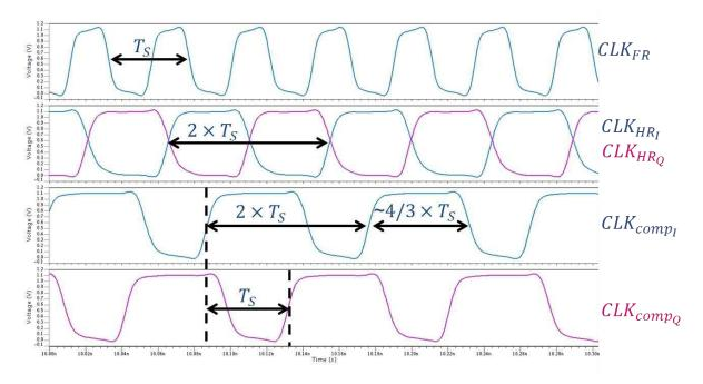
Figure 5-27: Clock generator simulation results
