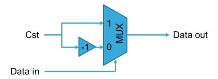
Figure 4-3: Multiplexer based multiplier
