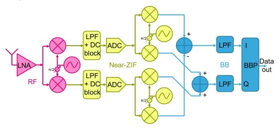
Figure 3-15: Near-ZIF receiver using the Weaver image cancelling approach with a digital implementation
