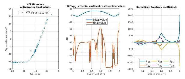
Figure 4-37: Optimization results for ELD values from 1 to 2  $T_S$
