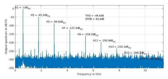
Figure 3-19: ADC output spectrum for a single tone input at  $-1dB_{FS}$
