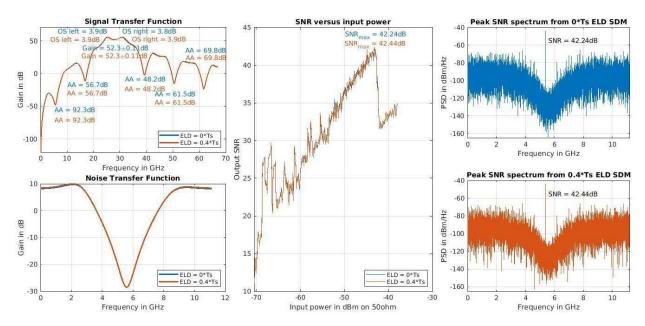
Figure 4-31: Comparison of modulators with respectively 0 and  $0.4 \times T_S$  ELD
