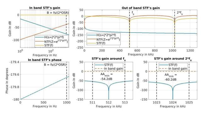
Figure 4-15: Signal Transfer Function characteristics of a first order LPCTSDM with an OSR of 256 and a bandwidth of 1kHz
