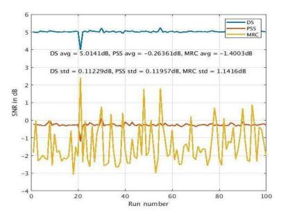
Figure 2-22: SNR for 100 channel realizations for DS, PSS and MRC beamforming
