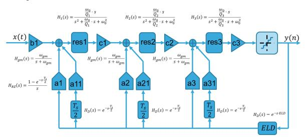
Figure 4-26: Modulator's architecture with its associated Laplace transforms
