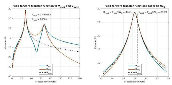
Figure 5-14: Feedforward transfer functions of a transformer-based resonator
