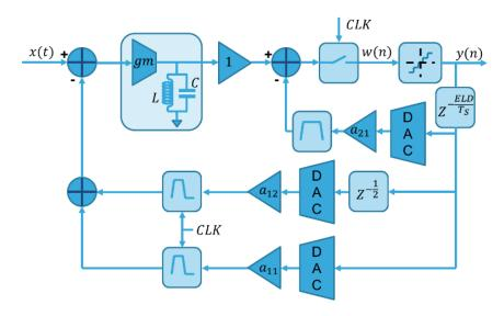
Figure 4-20: Modified BPCTSDM architecture for ELD compensation
