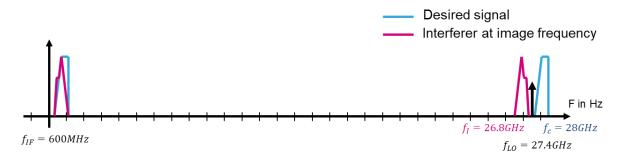
Figure 3-13: Impact of Image frequency on a Near-ZIF naive implementation
