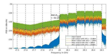
Figure 3-18: Output spectrum of the different building blocks for IIP3 compatible with MACLR specifications
