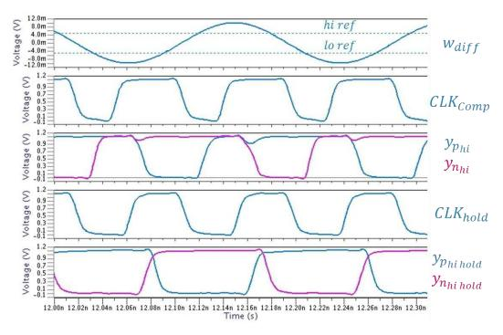
Figure 5-32: Simulation of the proposed latching comparator
