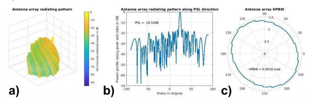
Figure 2-14: 364 elements MC-UCA a) Radiation Pattern b) Profile along PSL c) HPBW contour
