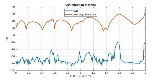
Figure 4-43: Optimizer final value and feedback coefficients' square sum
