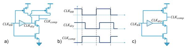
Figure 5-26: a) Classic pulse extender schematic. b) Pulse extender chronograms. c) Proposed pulse extender schematic
