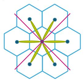
Figure 2-26: Distribution of backhaul links per sector for a cell division in four
