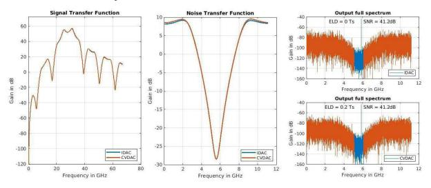
Figure 5-8: Comparison between an IDAC and CVDAC modulator after optimization
