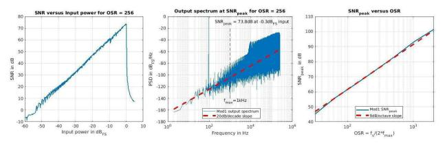
Figure 4-6: Simulation of a first order LPDTSDM. Left: SNR versus input power. Middle: Output spectrum at  $SNR_{peak}$ . Left:  $SNR_{peak}$  versus OSR
