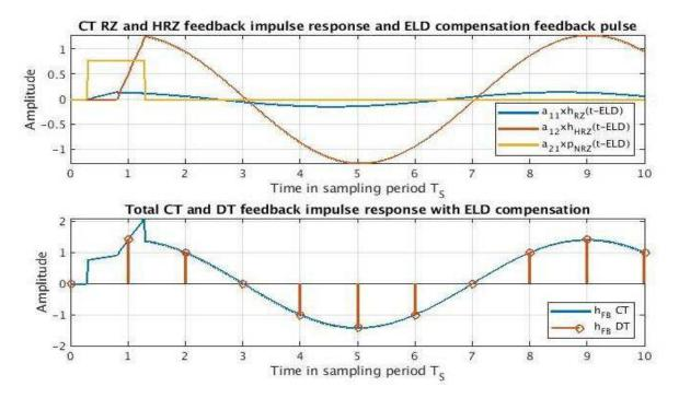
Figure 4-21: Feedback impulse response with ELD compensation
