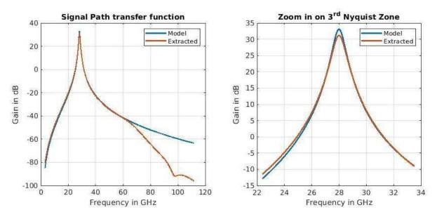
Figure 5-41: Signal Path transfer function from GSG input to comparator input
