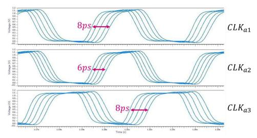
Figure 5-36: Delay elements tuning range  $\sim 187 \sim$
