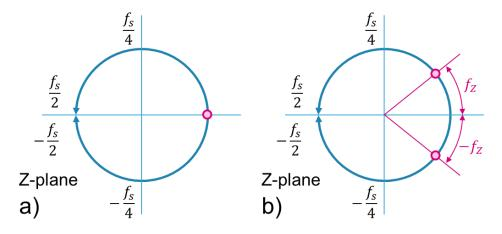
Figure 4-7: a) Zeros' location of a first order LPDTSDM. b) Zero locations of second order BPDTSDM
