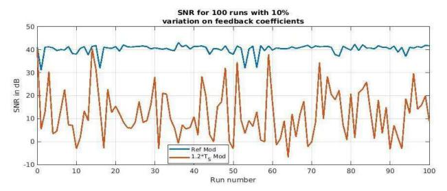
Figure 4-42: Reference and 1.2 clock cycle ELD modulators SQNR for Gaussian feedback coefficient varations over 100 runs
