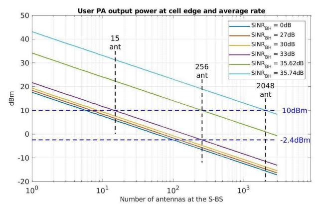
Figure 2-27: Users' PA output power at cell edge and average rate as a function of the number of receiving antennas for various  $SINR_{BH}$
