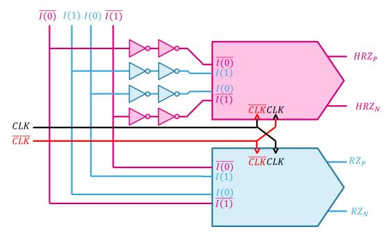
Figure 5-11: RZ and HRZ Voltage DAC assembly
