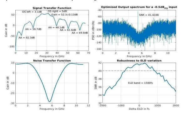
Figure 5-38: Initial LC based modulator perforamnces
