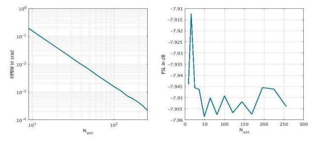
Figure 2-13: HPBW and PSL for UCAs versus the number of antennas Nant.
