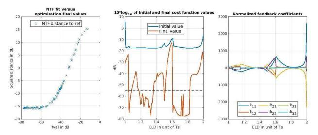
Figure 4-38: Optimization results for ELD values from 1 to 2  $T_S$  using previous point for initialization
