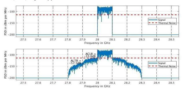
Figure 2-29: Impact of non-linearity on wide band signals. Top: original signal. Bottom: signal after undergoing non-linearity of third and fifth order
