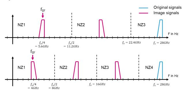
Figure 4-22: Frequency planning for a sampling frequency of 22.4GHz on top and 16GHz on the bottom
