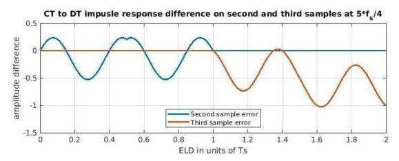
Figure 4-45: Second and third feedback impulse response sample errors versus ELD for a  $5 \times f_s/4$  second order BPCTSDM
