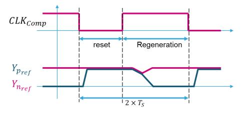
Figure 5-30: Clocked Comparator output chronogram
