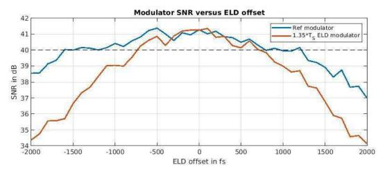
Figure 4-48: SNR versus ELD offset from -2ps to 2ps with a step of 100fs for the reference and  $1.35 \times T_S$  ELD modulators
