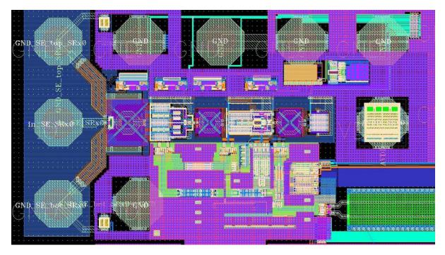
Figure 5-46: Single Receiver's layout
