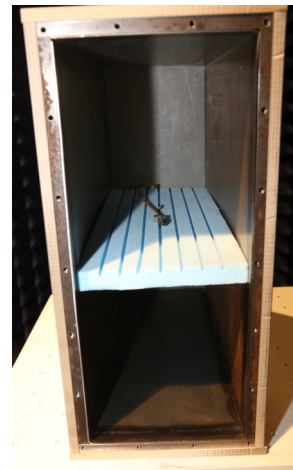
(b) Front view of the mock-up's main body with the electric gasket along the edges of the frame and the uniformly distributed screw threads.
