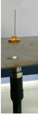
Fig. III.5.2 – A monopole attached to the front panel.
