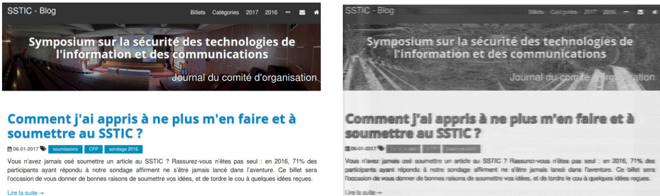
Fig. I.1.5 – Displayed image (left) and recovered image (right) from a DVI video stream (from [Ricordel and Duponchelle, 2018]).
