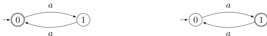
Figure 7: Two automata that are equivalent on infinite inputs but not on finite ones.
