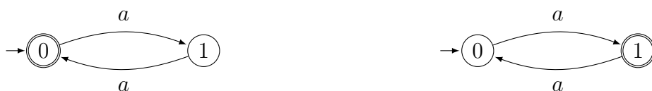
Figure 7: Two automata that are equivalent on infinite inputs but not on finite ones.
