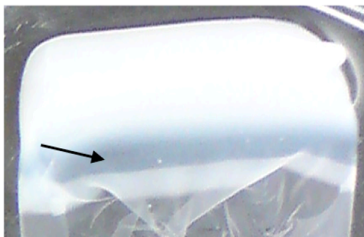
Fig. S1/ Matrix with a gradient in collagen concentration synthesized by slow evaporation. From top to down, the collagen concentration is increasing from 10 reaching 100 mg/mL. A gap in transparency (arrow) is observed inside the matrix and found at ~45 mg/mL after hydroxyproline titration.
