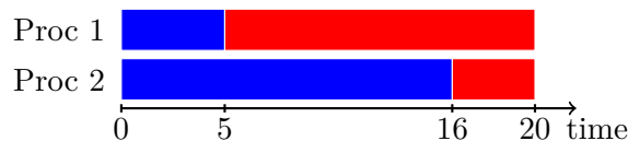
Figure 3.1: Toy example with two processors, two successfully completed tasks (in blue) and two not-yet-completed tasks (in red) at time 20.
