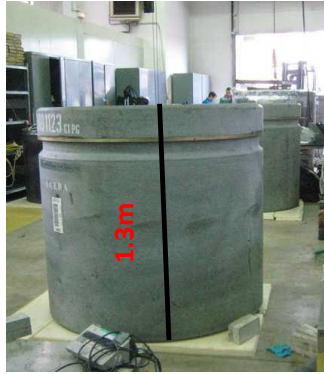
Fig. 1-1 – The C1PG SP nuclear waste package
