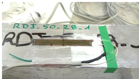
Fig. 4-23 – Deformation gauge placed on a sample used for drying shrinkage measurement
