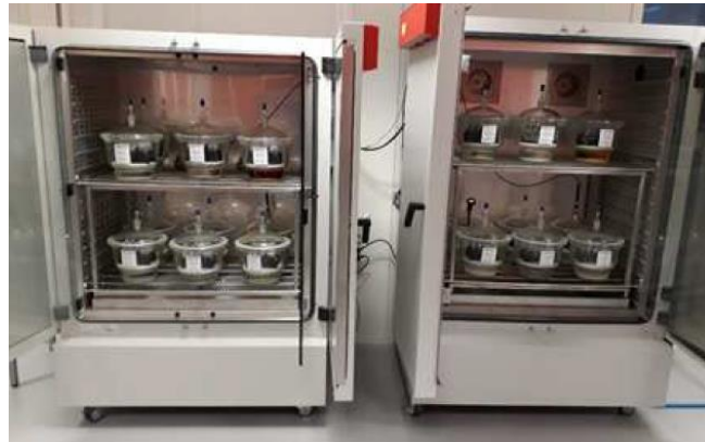
Fig. 2-21 – Two climatic chambers used to regulate temperature for the water vapor sorption tests
