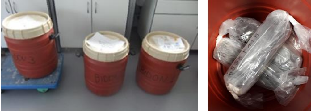
Fig. 2-19 – Autogenous conditioning of concrete samples
