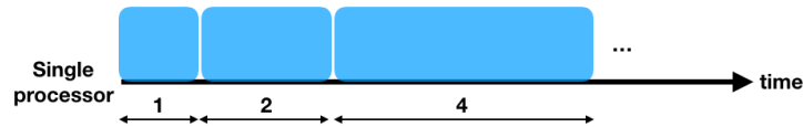
FIGURE 4.1 – A schedule of executions of the same algorithm in which the i -th execution time is 2^i .
