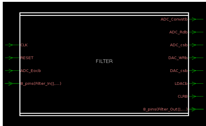
Figure 37: RTL (Top-level) view of FIR Filter
