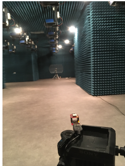
Figure 4.10: Screaming-channel attack at 10 m in an anechoic chamber.
