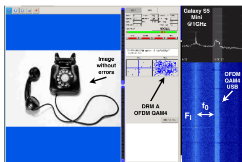
Figure 8.2: Example of digital image transmission using HamDRM (OFDM, QAM 4 , error correction) on a Samsung Galaxy S5 Mini . The signal, modulated in amplitude and phase, is sent in SSB at 1 GHz \pm 9.6 kHz.
