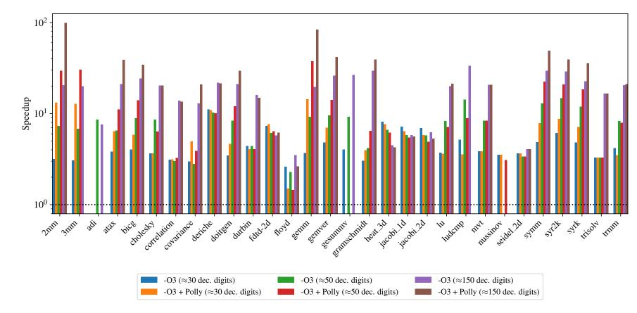
Figure 6.5: Speedup of vpfloat<unum, ...> over vpfloat<mpfr, ...> on the PolyBench suite
