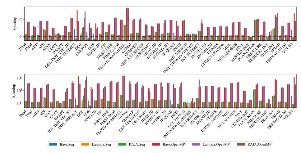
Figure 6.4: Speedup of vpfloat<mpfr, ...> over the Boost library for multi-precision for the RAJAPerf benchmark suite, both compiled with -O3 optimization level.
