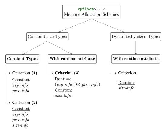
Figure 4.3: Memory Allocation Schemes for Constant-Size and Dynamically-Sized Types
