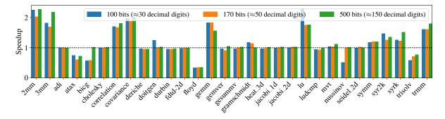
Figure 6.1: Speedup of Polly's loop nest optimizer in Polybench compiled for vpfloat<mpfr, ... types.
