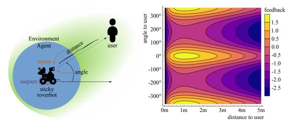
Figure 1.1: Left: The imaginary sticky roverbot used as an example learning agent in this chapter. Right: Contour plot of an example feedback profile for the roverbot, defined with respect to the user distance and angle.
