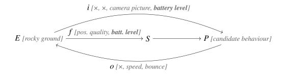
Note that a new battery sensor has also been added (+i).
