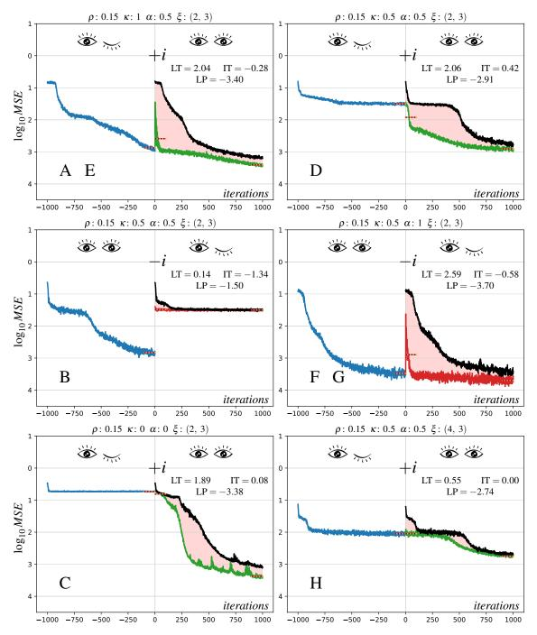
Figure 6.2: Learning curves *l*: evolution of MSE for key example individual runs in the experiment illustrating the observed effects A, B, C, D, E, F, G and H (Section 6.8). Filled areas illustrate the LT measure (7.85). Dotted bars illustrate the IT measure (7.87) and the LP measure (7.88). The eyes represent 1D/2D input signatures. The signature change event occurs at time 0.
