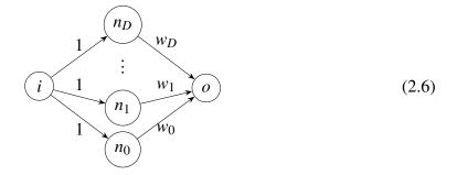
In this representation, node labels represent functions, and arrow labels represent weights. The value of each arrow tip is the value of its source node multiplied by its label, and the value of each node (or "neuron") is the sum of incoming arrows tips transformed by the node label. Here, i and o correspond to identity functions, in particular, *input* and *output* of the procedure, while each  $n_d$  is the power function:
