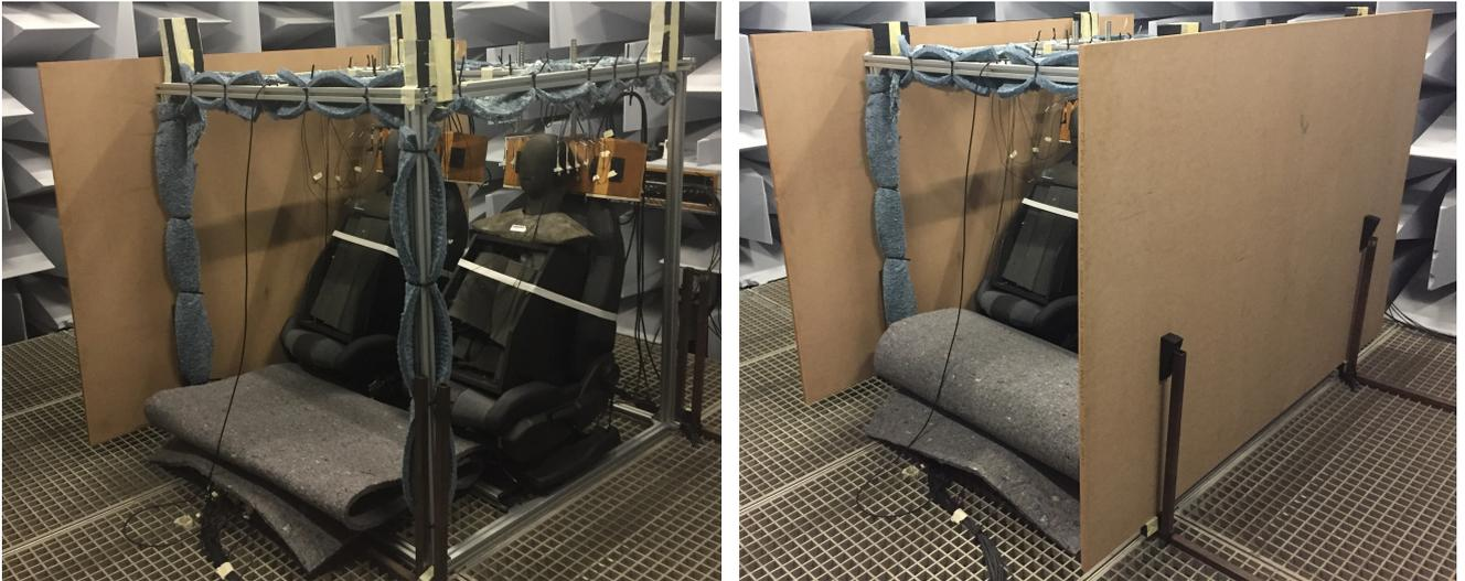
Figure 3.25: Prototype in the anechoic chamber with reflective panels.
