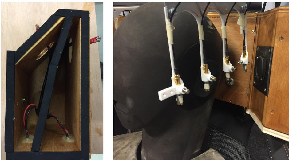
Figure 3.13: Prototype: Loudspeaker enclosure top view (left), seat close up (right).
