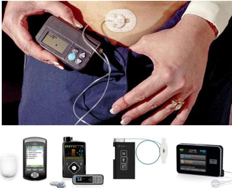
**Figure 5:** Insulin pump panel and use. External insulin pump delivering subcutaneously in the abdomen of a patient (up). A representative panel of off-the-shelves insulin pump (down). Omnipod®, Minimed™ 640G, Ypsopump™, Tandem t-slimX2™ (from left to right).
