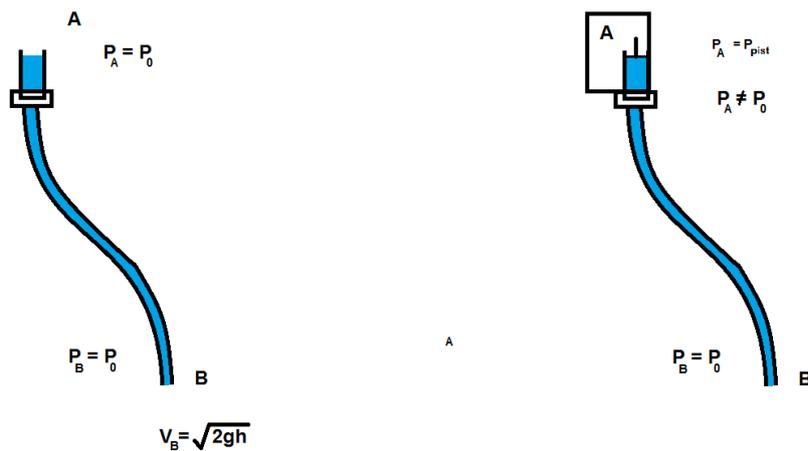
**Figure 14:** Siphon effect phenomenon adapted to CSII. Hydrostatic effect situation with an open reservoir (left) and with reservoir inside an CSII (left).
