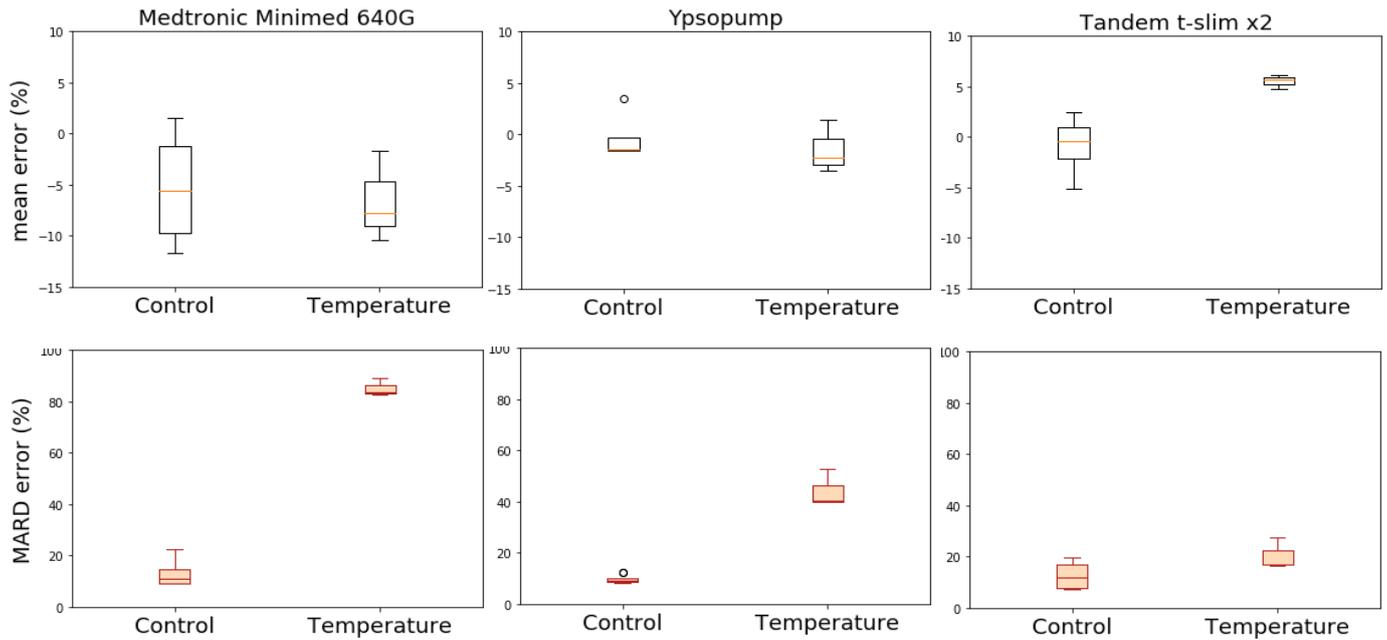
**Figure 19:** Pump delivery error for temperature variations. MARD (down) et mean (up) delivery error boxplot for Medtronic® Minimed™ 640G (left), Ypsopump™ (middle) and t:slimX2™ (right).
