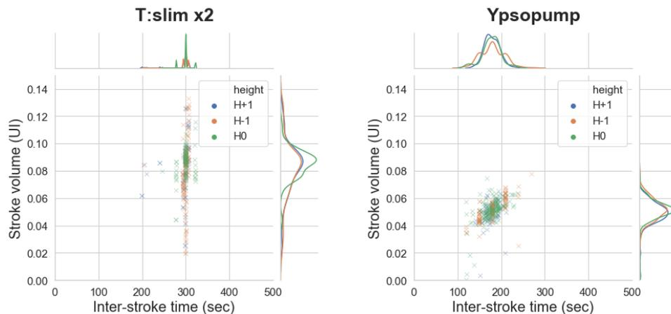
**Figure 17:** Peak-wise analysis of pump precision for hydrostatic pressure conditions. Tandem t:slimX2™ (right) and Ypsopump™ (left) insulin stroke delivery parameters (volume and frequency) were compared for each hydrostatic pressure conditions.
