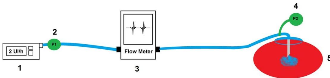
**Figure 25:** Back pressure distribution for CSII delivery setup. An CSII (1) delivers within a swine skin tissue (5). Pressure profiles is measured out of the pump (2) and before injection site (4). Flow rate is also considered (3).
