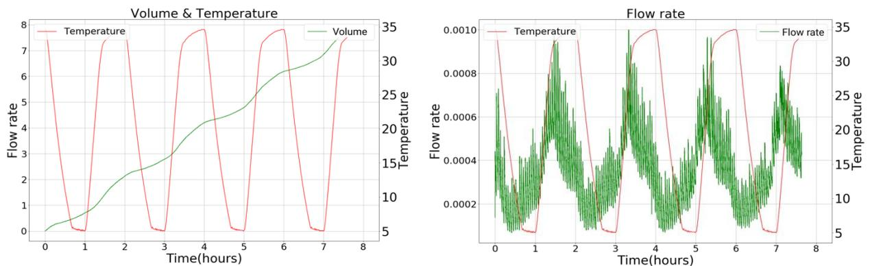
**Figure 20:** Flow rate and volume of CSII delivery following temperature variations. Temperature variations (red) from 5°C to 35°C is correlated with volume (green – left) and flow rate (green - right) CSII delivery.
