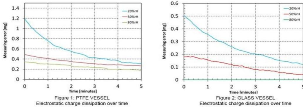
**Figure 10:** Electrostatic weighing disruption phenomenon. Electrostatic charge dissipation over the time likely to cause vicious and hardly detectable measurement drift. (Source: <https://www.mt.com/in/en/home/library/collections/laboratory-weighing/electrostatic-and-weighing.html>)
