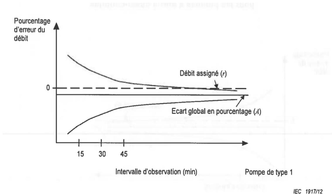
**Figure 9:** CSII assessment trumpet curve. Pump flow rate percentage error consider over several observation windows.
