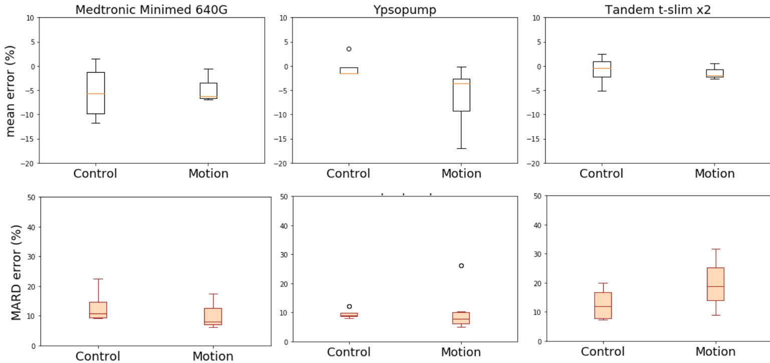
**Figure 24:** CSII global error delivery under motion constraint. MARD (down) and mean (up) distribution of Medtronic® Minimed™ 640G (left), Ypsopump™ (middle) and Tandem t:slimX2™ (right). Comparison of MARD error distribution without motion (control) versus with motion.
