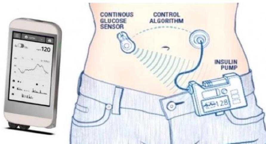
**Figure 7:** Artificial pancreas system description. CGMS and CSII plugged in subcutaneous tissue and combined with a control algorithm that automatically calculate insulin dose to inject. (Source: <https://www.medgadget.com/>)
