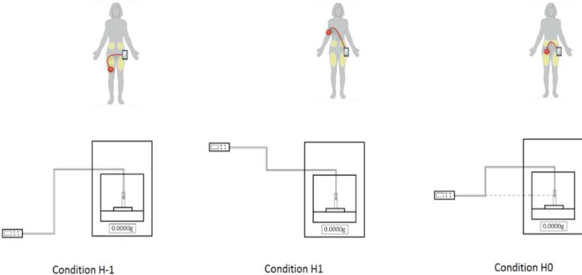
**Figure 15:** Setup relative to each height conditions. Photo setup example in configuration H1 (up) and scheme describing test conditions with: condition H-1 model pump upward situation (left), condition H1 model pump downward situation (center) and condition H0 model control situation with no height difference (right).
