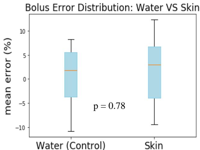
**Figure 27:** Bolus error distribution: skin injection vs in-water injection. 2UI boluses were infused within skin tissue (right) and water reservoir (left) end points. Delivery error distribution for each situation based on flow rate measurement integration were compared.
