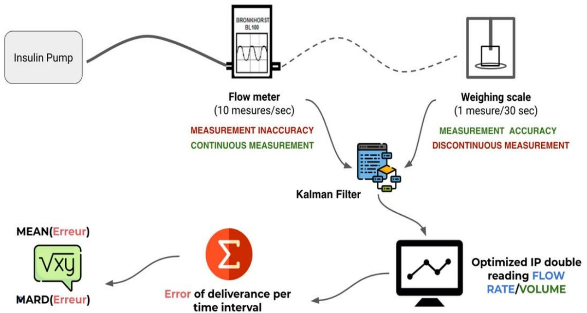
**Figure 12:** Novel methodology setup. Kalman filter-based double reading of insulin volume and flow rate using. CSII errors are then analyzed using MARD and mean indicators.
