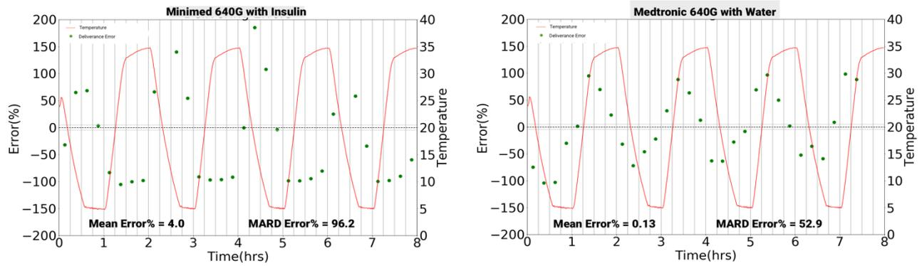
**Figure 21:** CSII delivery error under temperature constraints with insulin versus water. 15-minutes time interval delivery errors are calculated along experiment. Based on examples of Minimed™ 640G tests, we compare temperature variations constraint on CSII accuracy using water (right) and insulin (left).
