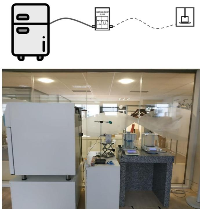
**Figure 18:** Testing setup for CSII precision assessment under temperature constraint. CSII is placed inside a programmed incubator that change temperature from 5°C to 15°C every hour. CSII flow rate is assessed using the KF-based double reading bench test.
