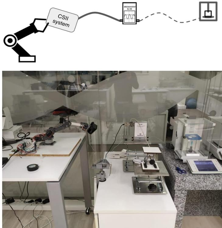
**Figure 23:** Testing setup for CSII precision assessment under motion constraint. CSII is stuck to an Arduino-based 6-axis robot arm that moved according to pre-programmed motions. CSII
