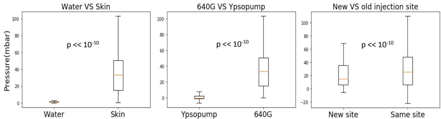
**Figure 28:** Down Stream pressure distribution. Pressure distribution comparison between an intra-skin and in-water reservoir (left), 640G and Ypsopump™ CSII model (middle) and within a novel injection
