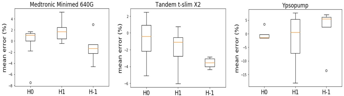
**Figure 16:** CSII delivery error under hydrostatic pressure constraint. Pourcentage of each test's mean error for Tandem t:slimX2™, Ypsopump™ and Minimed™ 640G at each height conditions (H0, H1,H-1)
