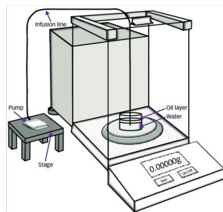
**Figure 8:** IEC 60601-2-24 standard protocol setup. Indirect insulin flow rate measurement based on a time-stamp micro gravimetric method. (Source: Bowen et al, 2016)
