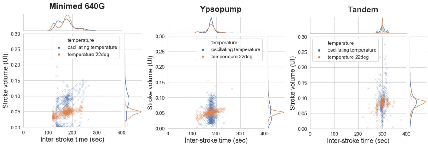
**Figure 22:** CSII delivery stroke analysis under TV conditions. Volume delivered for each stroke as well as time between each stroke is compared for CSII with (red) and without (blue) TV constraint for Minimed<sup>®</sup> 640G (left), Ypsopump<sup>™</sup> (middle) and Tandem t:slimX2<sup>™</sup> (right).
