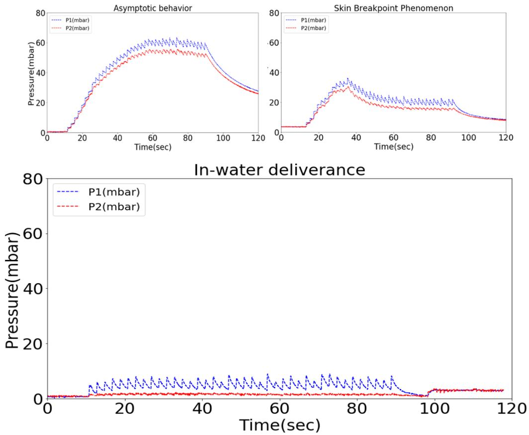
**Figure 26:** Up stream and down stream pressure time-series example of CSII infusion within skin tissue (up) and within water reservoir (down). Identification of two intra-skin pressure delivery: asymptotic pressure behavior (up left) and skin breakpoint phenomenon (up right).
