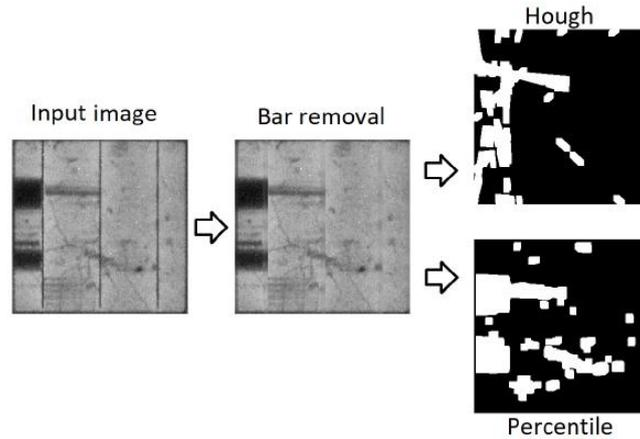
Figure II-5 Illustration of feature extraction from PV EL images [55]
