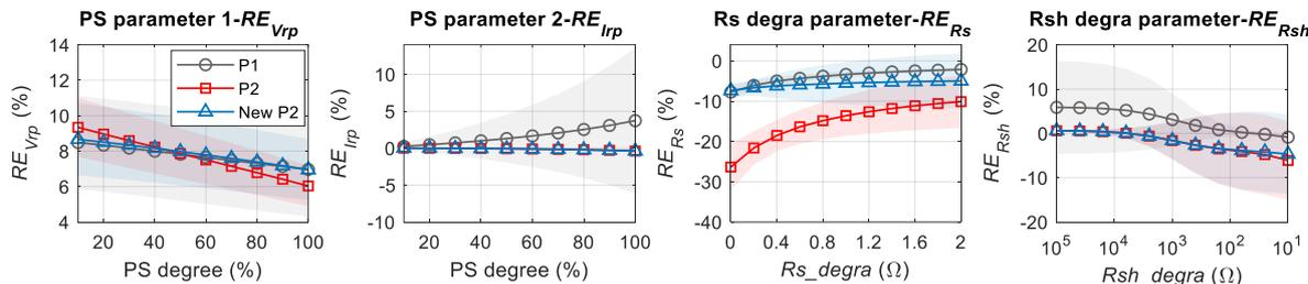
Figure III-15: *RE* of fault parameters under PS,  $R_s$ , and  $R_{sh}$  degradations with variable fault severity
