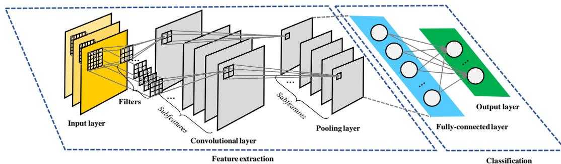
Figure II-9 Basic architecture of CNN
