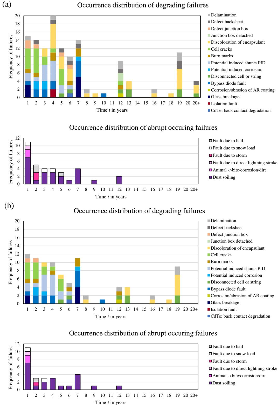
Figure I-5: Occurrence distribution of PV faults over years [56]
