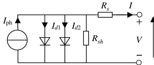
Figure II-3 Equivalent circuit of the two-diode model
