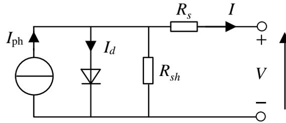
Figure II-2 Equivalent circuit of the single-diode model
