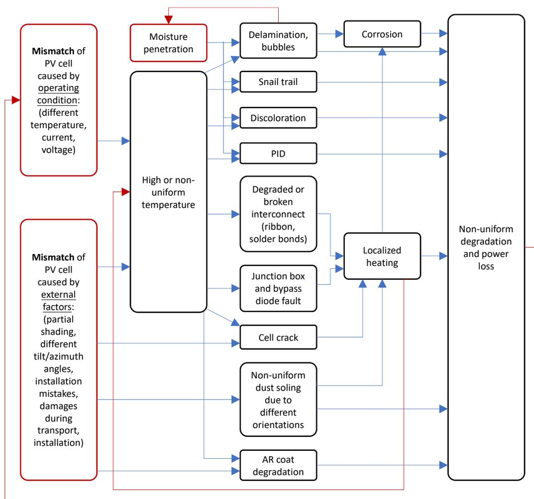
Figure I-2: Cause-effect circle between mismatch and degradation [38]
