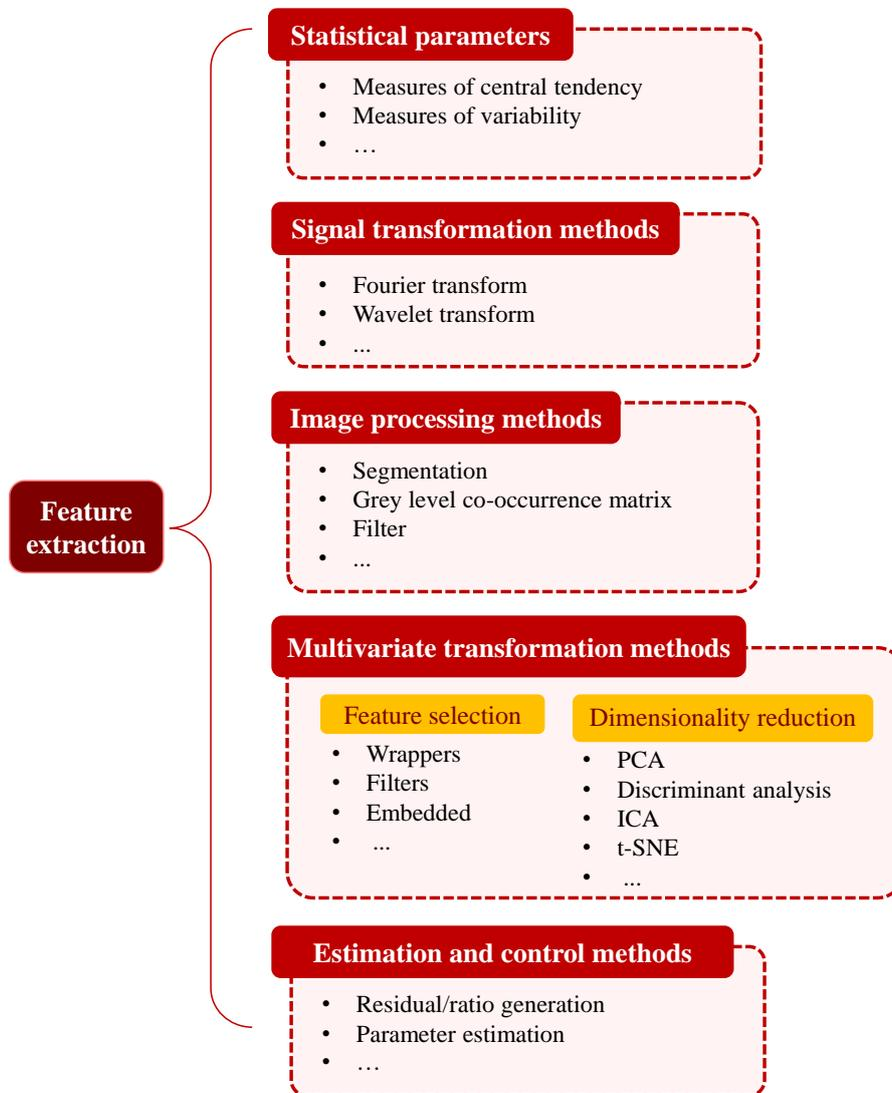
Figure II-4 Common techniques of feature extraction for FDD
