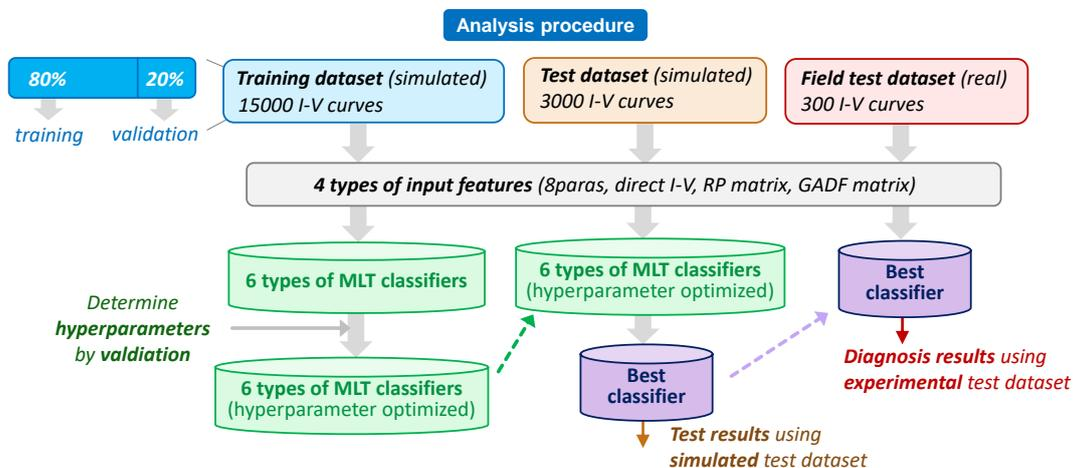
Figure IV-10: Feature analysis procedure
