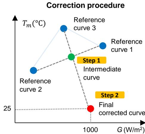
Figure III-6: Illustration of two-step correction procedure with three curves on  $T_m(G)$  plot
