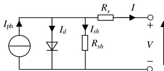
Figure III-1: Electrical equivalent circuit of single diode model
