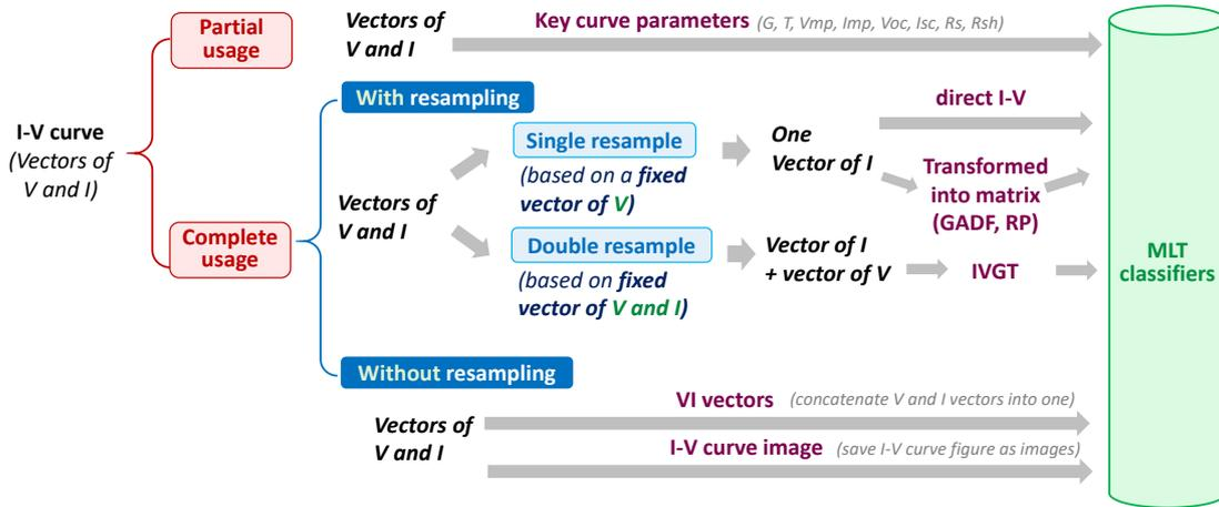
Figure IV-32: Feature extraction methods of I-V curve for comparison study
