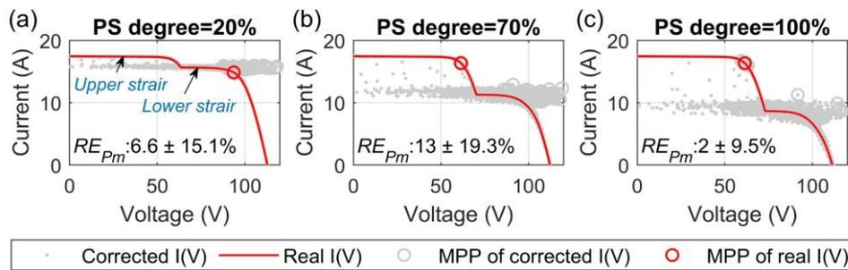
Figure III-22: Corrected curves using P3 under three fault severities of PS
