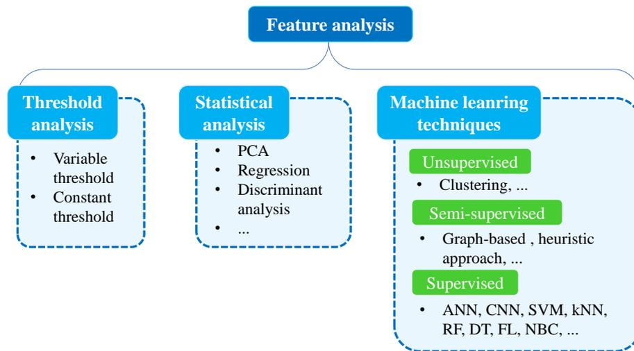
Figure II-7 Techniques for feature analysis in FDD
