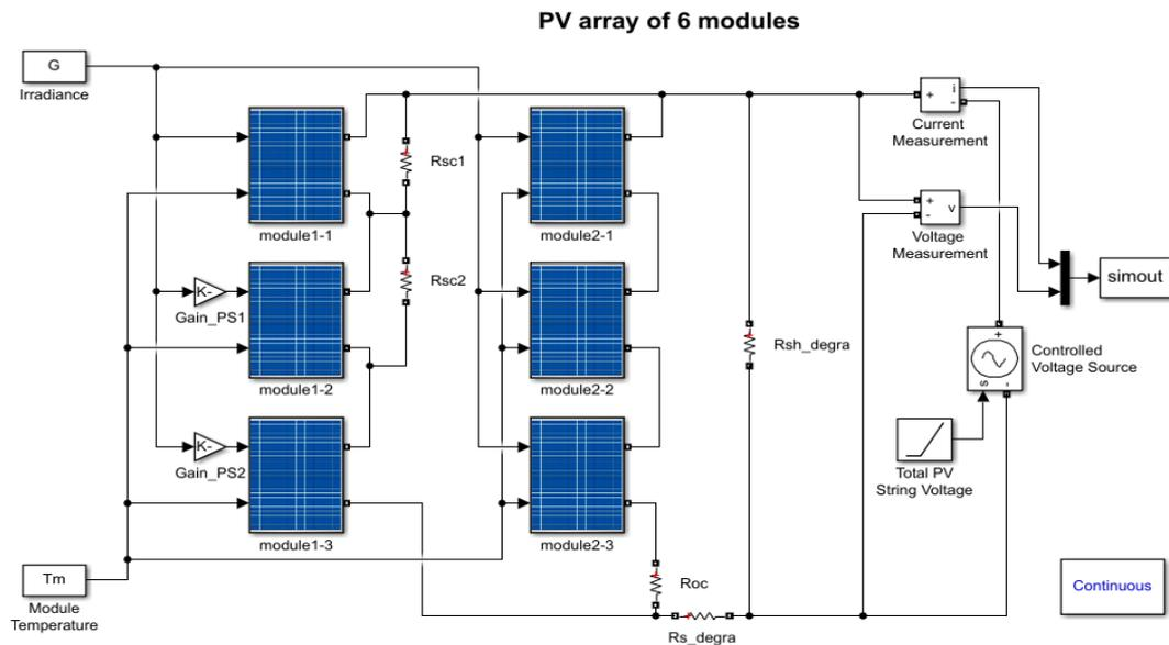
Figure IV-1: Simulation model of the PV array
