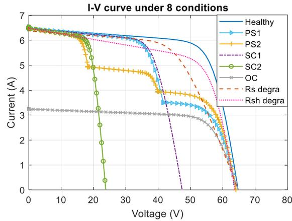
Figure IV-2: Examples of simulated I-V curves under 8 PV array conditions
