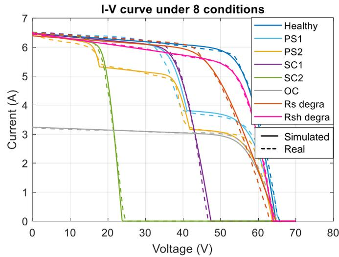
Figure IV-30: Examples of corrected real and simulated I-V curves
