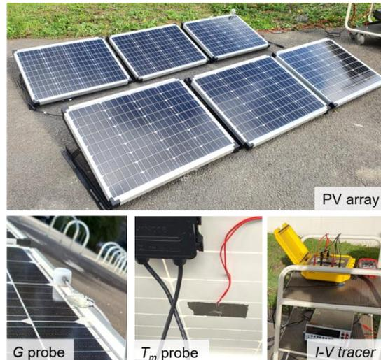
Figure IV-28: Field test setup
