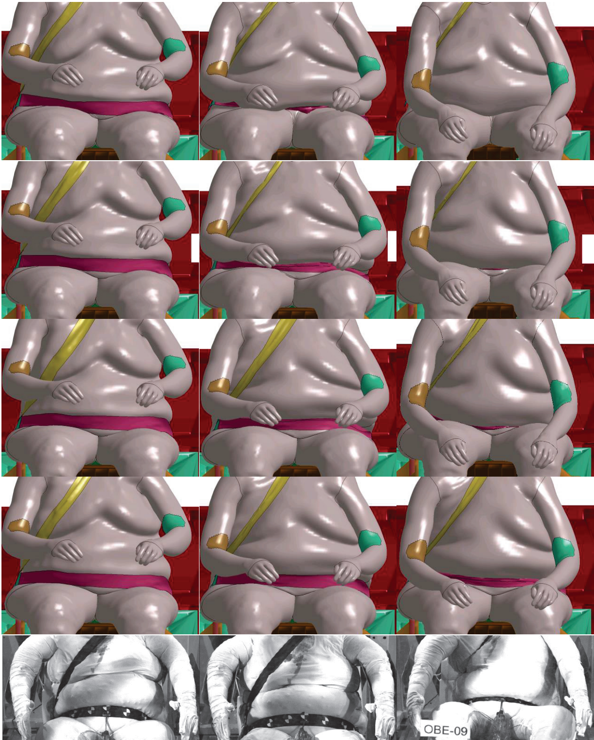
Figure 116: Frontal view of the MS743 sled simulation at 30 ms (left), 60 ms (middle) and 90 ms (right). Each row shows a simulation with different friction, from top to bottom: 0.3, 0.5 and 0.8, all with the C315 material. Fourth row shows the simulation with friction 0.8 and the X1 material, although the third image is from time 79 ms as the simulation terminated afterwards due to negative volume elements. Last row shows the PMHS experiment.
