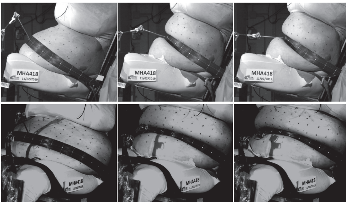
Figure 35: Side and corner view (front camera data were corrupted) of the MHA418 experiment at three points of interest. Left: initial position (time 0 ms). Middle: maximum belt force. (120.5 ms). Right: maximum centre resultant displacement (146.5 ms).
