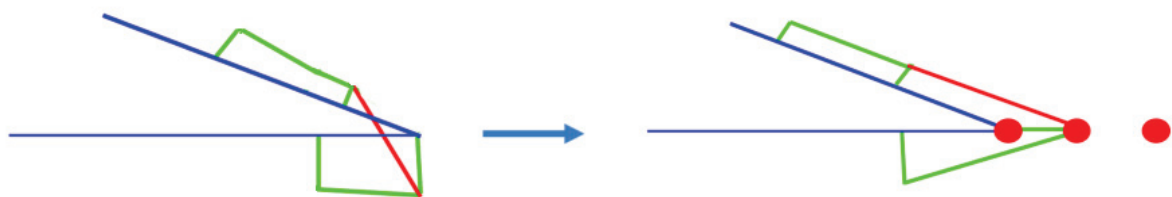
Figure 79: Schematic representation of the fold as a sharp angle (Skin in blue, inner soft tissues elements in green and red). Left: penetrations resulting from Kriging without controlling for the sharp angle. Right: the folding line is enforced by additional control points (red dots) on the skin and inside the tissues.
