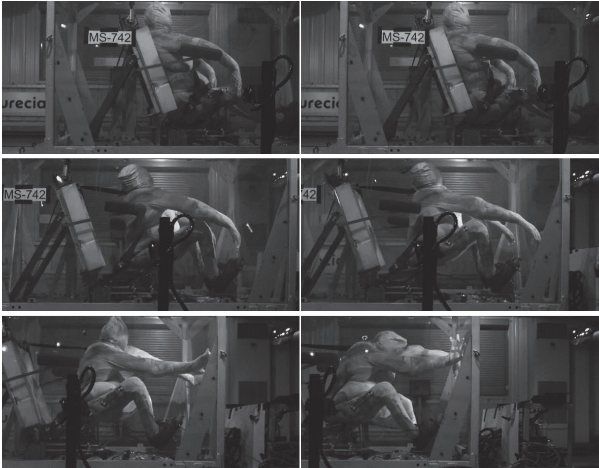
Figure 43: Right camera footage from sled tests with MS742. Top left: initial position (time 0 ms). Top right: end of pretension phase (40 ms). Middle left: peak buckle force (87.5 ms). Middle right: peak lap belt anchor force (99 ms). Bottom left: unloading, 120 ms. Bottom right: unloading, 140 ms.
