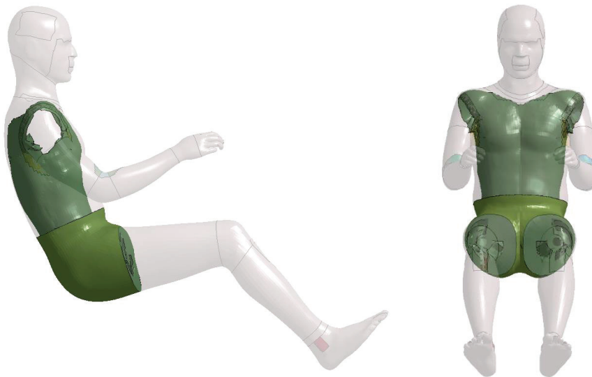
Figure 81: Subcutaneous fat and abdominal muscles of the GHBM-M50-O combined to a single tetrahedral part (in green). The fascia of the abdominal muscles were kept on their posterior aspect and their thickness doubled to account for the muscle removal.
