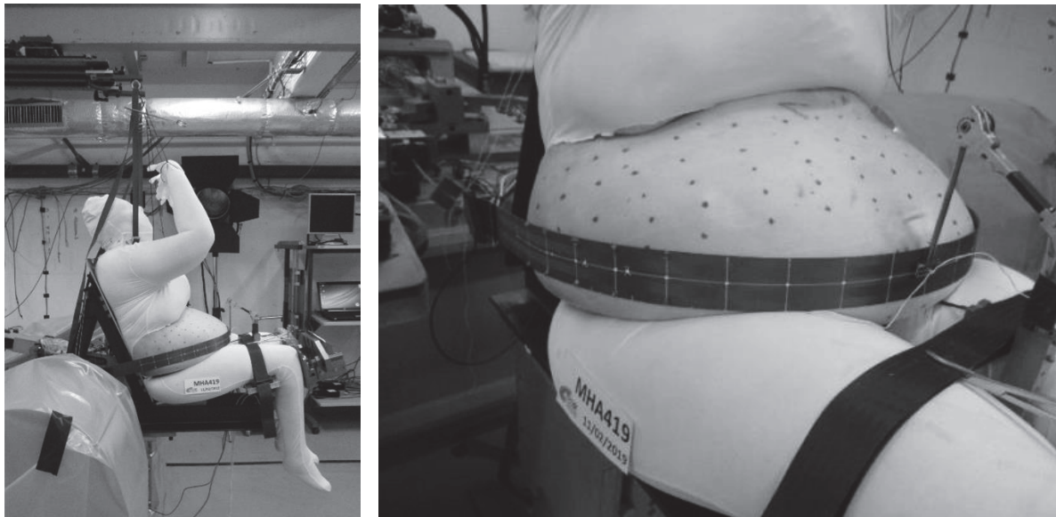
Figure 29: Illustration of the belt test setup for the parallel configuration. A custom device (called MP2D) used to measure the displacement on the centre of the abdomen can be seen on the right side of the right photo.
