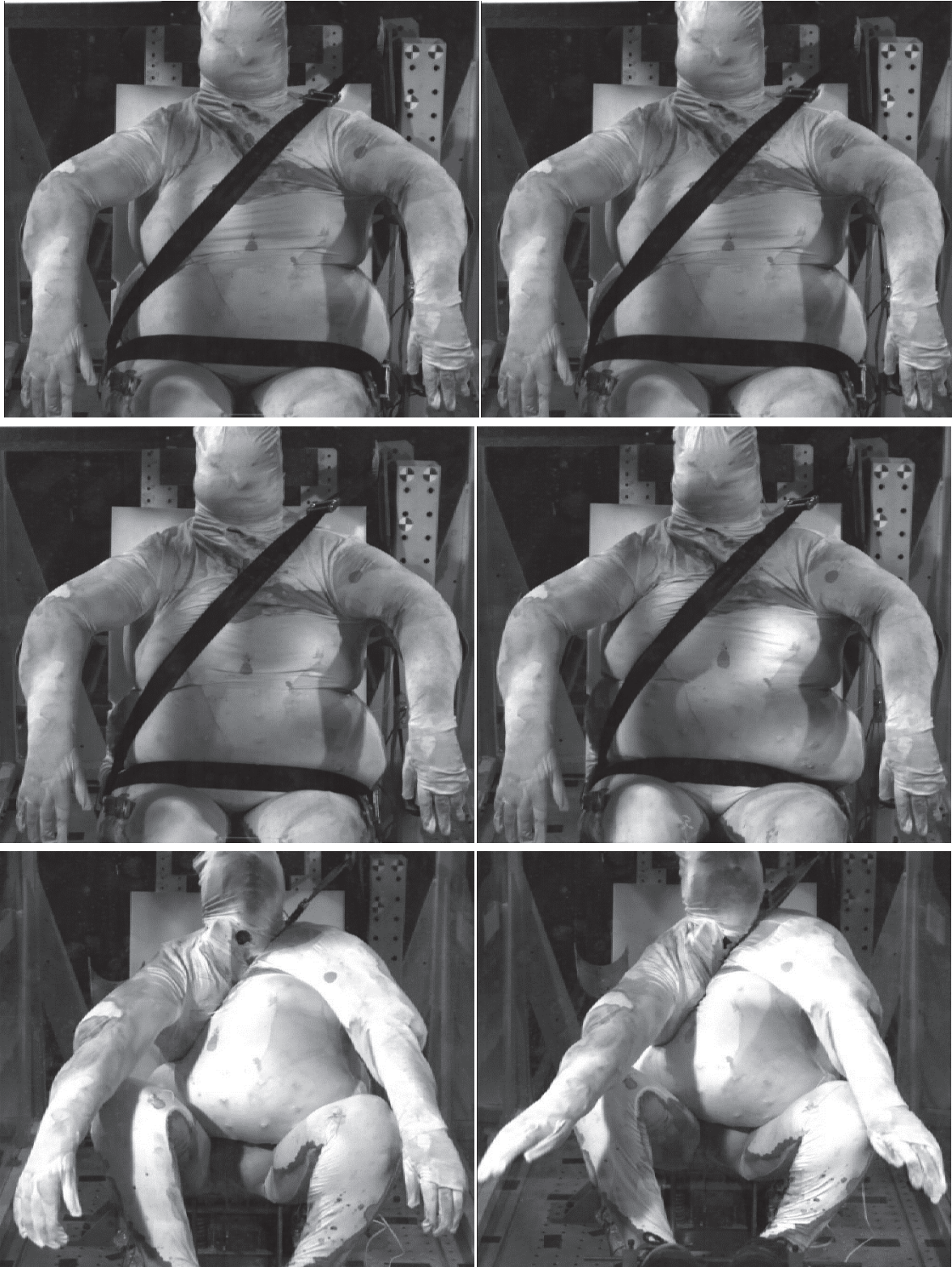
Figure 45: Front camera footage from sled tests with MS742. Top left: initial position (time 0 ms). Top right: 2 ms after PT1 was triggered (20 ms). Middle left: 2 ms after PT2 was triggered (27 ms). Middle right: end of pretension phase (40 ms). Bottom left: peak buckle force (87.5 ms). Bottom right: peak lap belt anchor force (99 ms).
