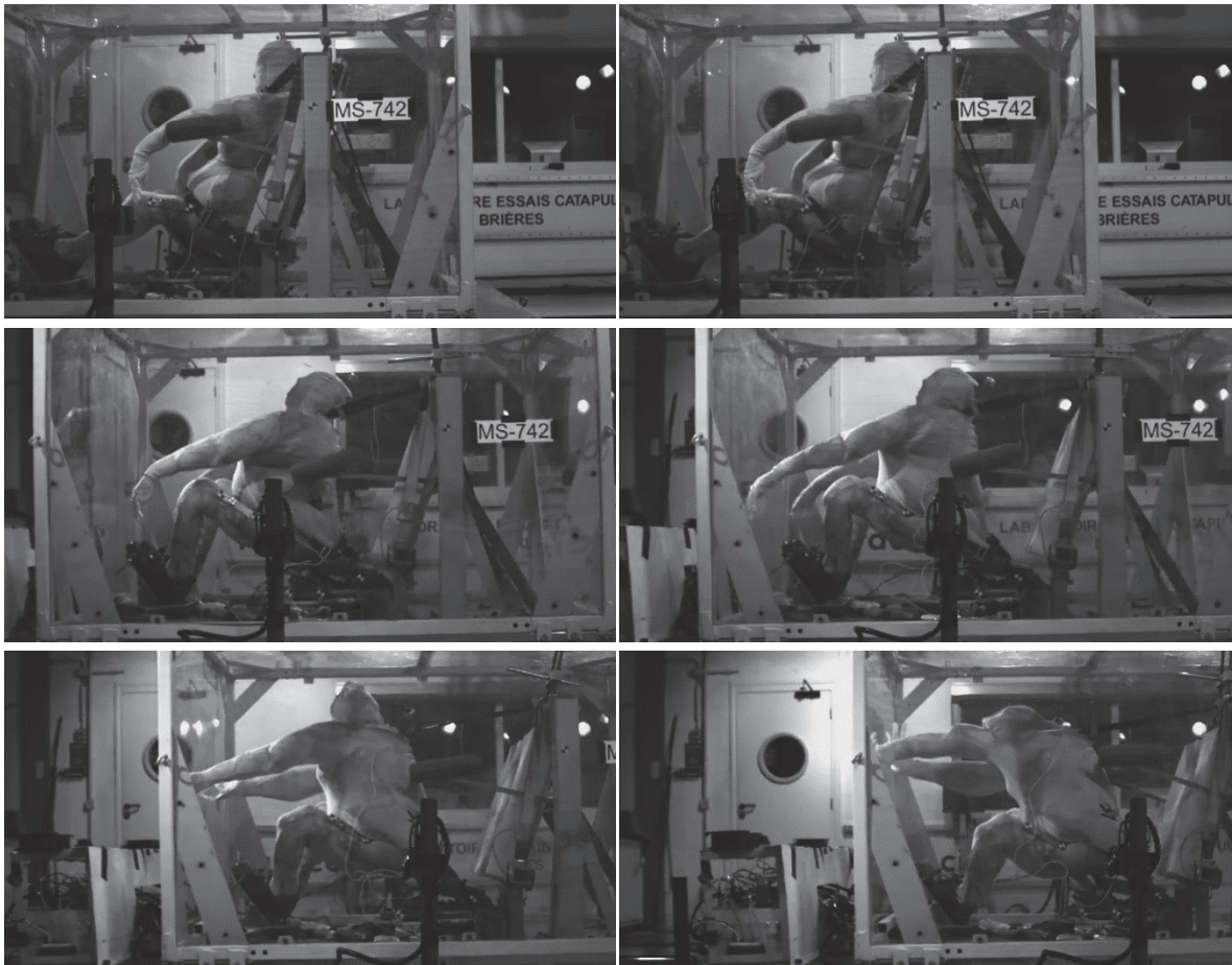
Figure 44: Left camera footage from sled tests with MS742. Top left: initial position (time 0 ms). Top right: end of pretension phase (40 ms). Middle left: peak buckle force (87.5 ms). Middle right: peak lap belt anchor force (99 ms). Bottom left: unloading, 120 ms. Bottom right: unloading, 140 ms.
