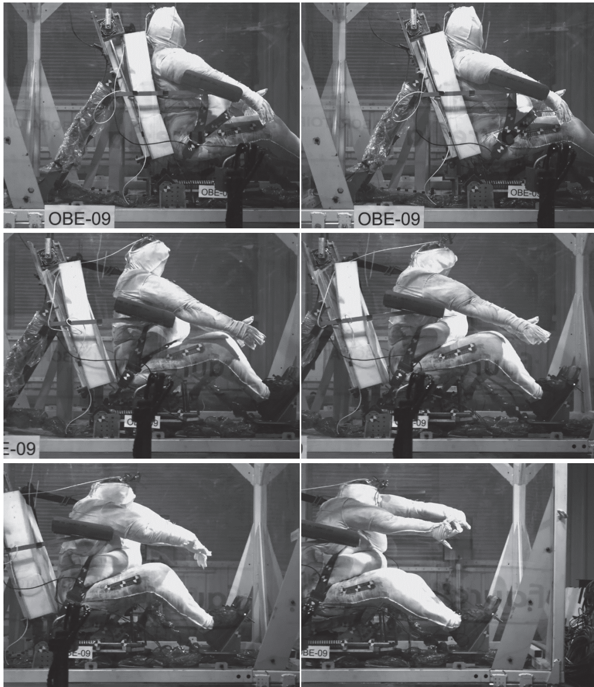
Figure 46: Right camera footage from sled tests with MS743. Top left: initial position (time 0 ms). Top right: end of pretension phase (40 ms). Middle left: peak buckle force (96.5 ms). Middle right: peak lap belt anchor force (111.5 ms). Bottom left: unloading, 130 ms. Bottom right: unloading, 160 ms.
