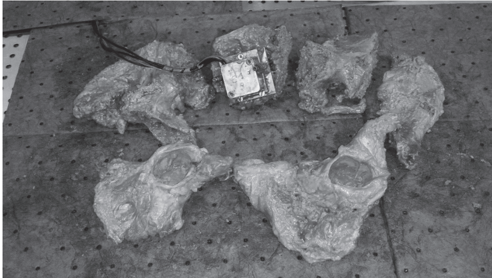
Figure 32: Fractured pelvis of the MS742 PMHS after the sled test.
