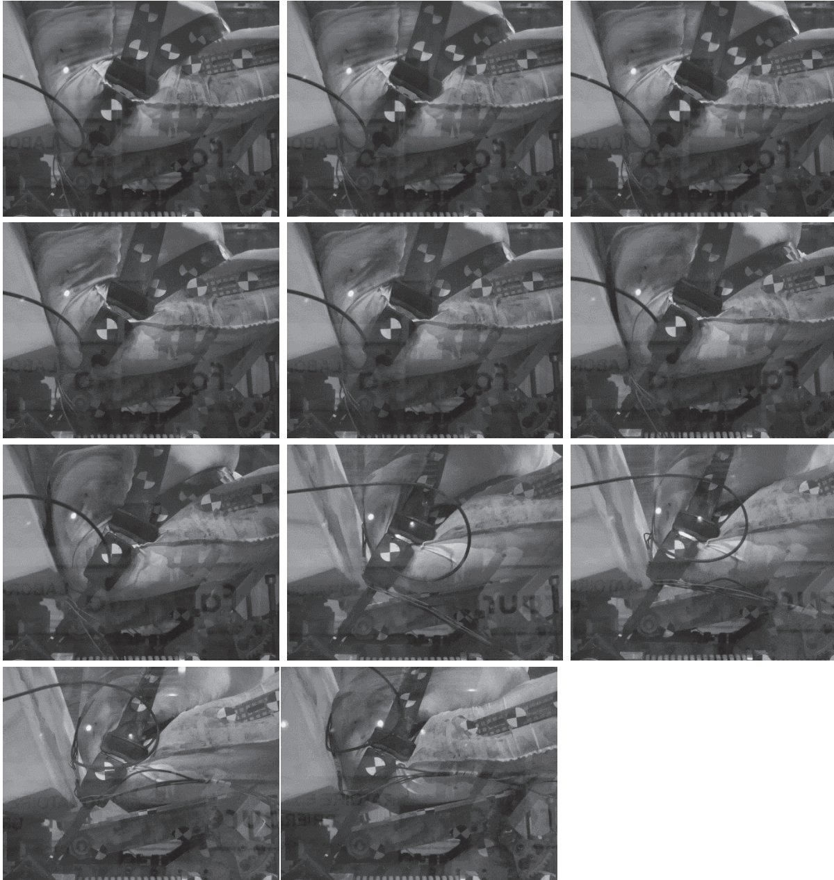
Figure 49: Buckle camera footage from sled tests with MS743. Images are in chronological order from left to right, top to bottom: initial position (time 0 ms), PT1 triggers (18 ms), 2 ms after PT1 was triggered (20 ms), PT2 triggers (25 ms), 2 ms after PT2 was triggered (27 ms), end of pretension phase (40 ms), start of main loading phase (50 ms), peak buckle force (96.5 ms), peak lap belt anchor force (111.5 ms), unloading (130 ms), unloading (160 ms).
