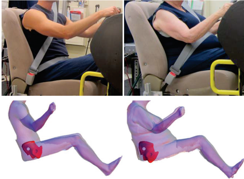
Figure 11: A side view of non obese (left, BMI 23) and obese (right, BMI 31) vehicle occupants illustrating the different conditions for placing the lap belt. The bottom row shows mesh obtained from surface scans of the volunteers shown on the top row. Images provided by Jingwen Hu, Jonathan D. Rupp, Matthew P. Reed (University of Michigan, Transportation Research Institute).
