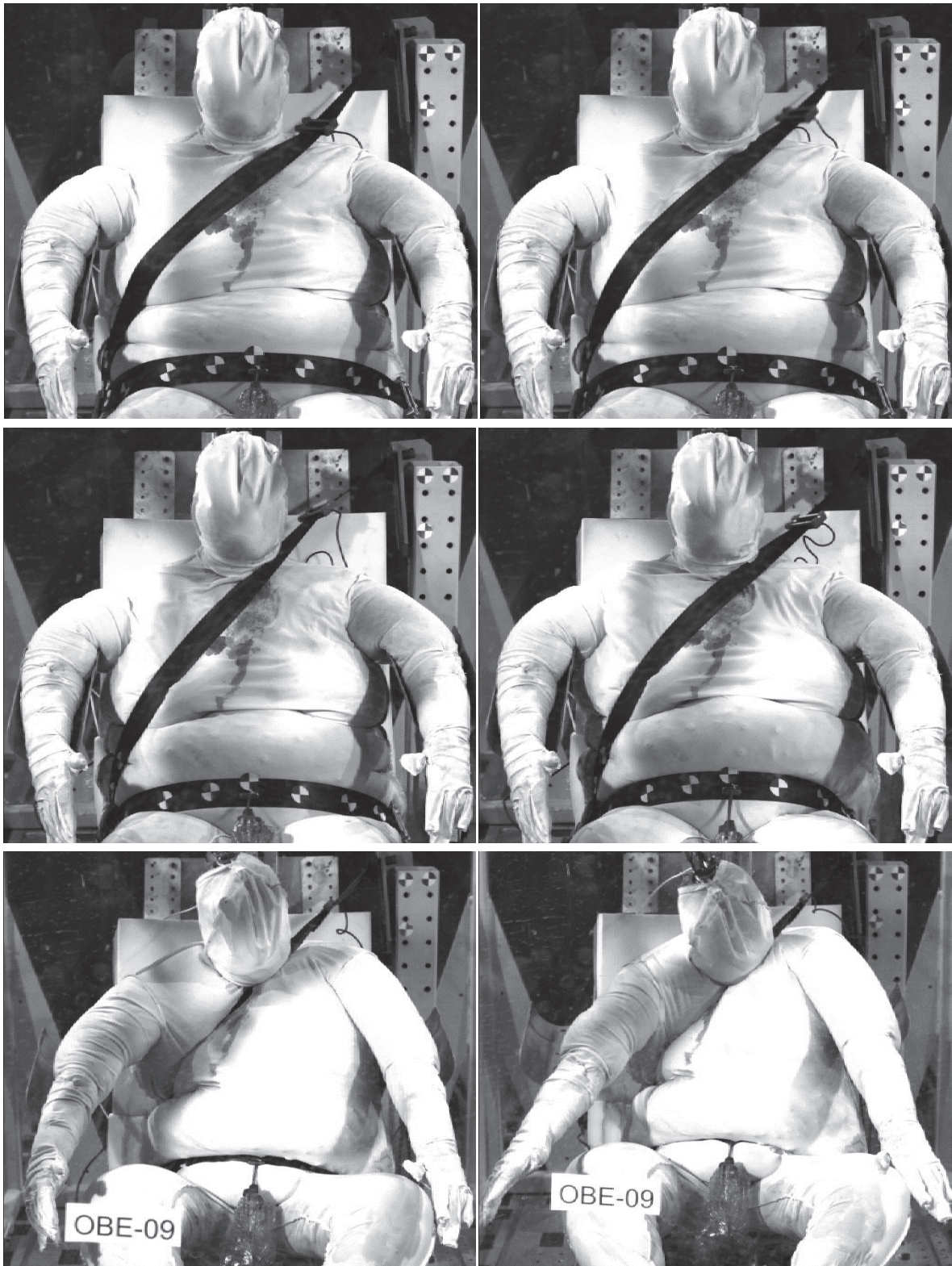
Figure 48: Front camera footage from sled tests with MS743. Top left: initial position (time 0 ms). Top right: 2 ms after PT1 was triggered (20 ms). Middle left: 2 ms after PT2 was triggered (27 ms). Middle right: end of pretension phase (40 ms). Bottom left: peak buckle force (96.5 ms). Bottom right: peak lap belt anchor force (111.5 ms).
