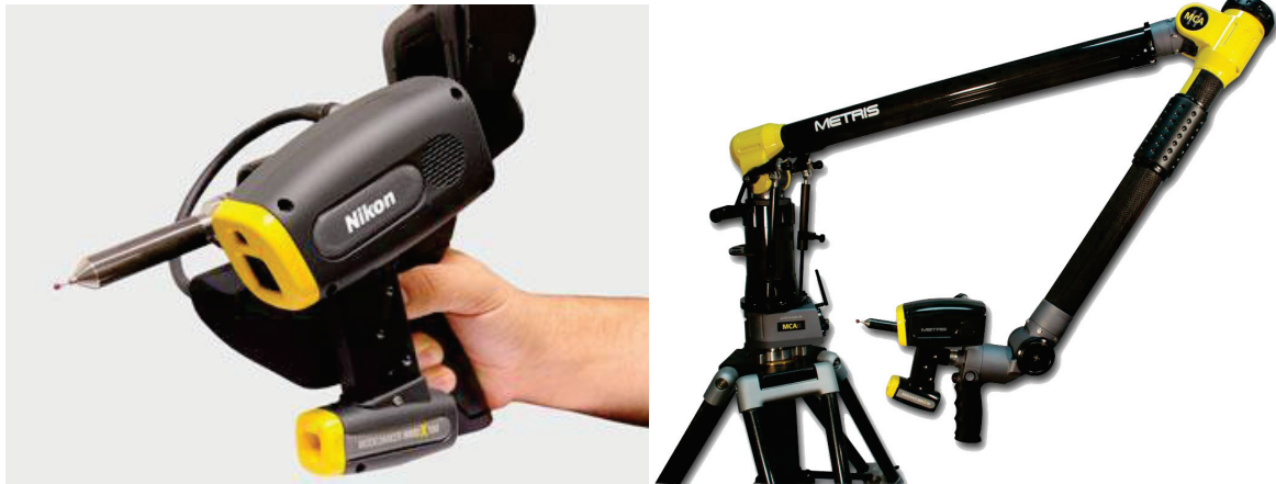
Figure 26: The laser scanner (left) and measuring arm (right) used for surface scanning. Image source: www.nikonmetrology.com (left), metrisusa.wordpress.com (right), accessed May 2020.
