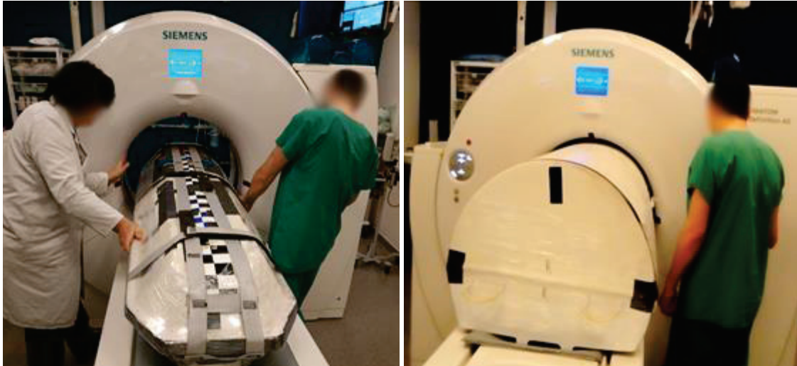
Figure 24: CT scanning of the PMHS. Left: smaller container for supine posture with arms crossed. Right: larger container for the other postures.
