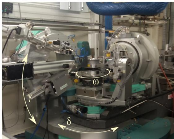
Figure 3.4: The picture of the ID10 beamline with the rotation angles displayed. The horizontal angle called  $\delta$  and the vertical is called  $\gamma$ .  $\omega$  is the rotation angle around the  $\hat{z}$  axis.
