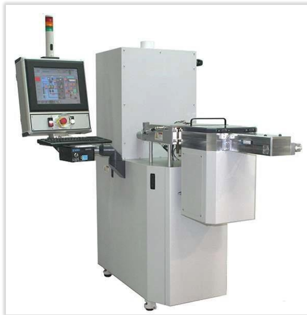
Figure II-33 : HF Vapor Release Etch from Primaxx® Monarch 3 with an integrated Panel PC in PTA-Grenoble cleanroom.
