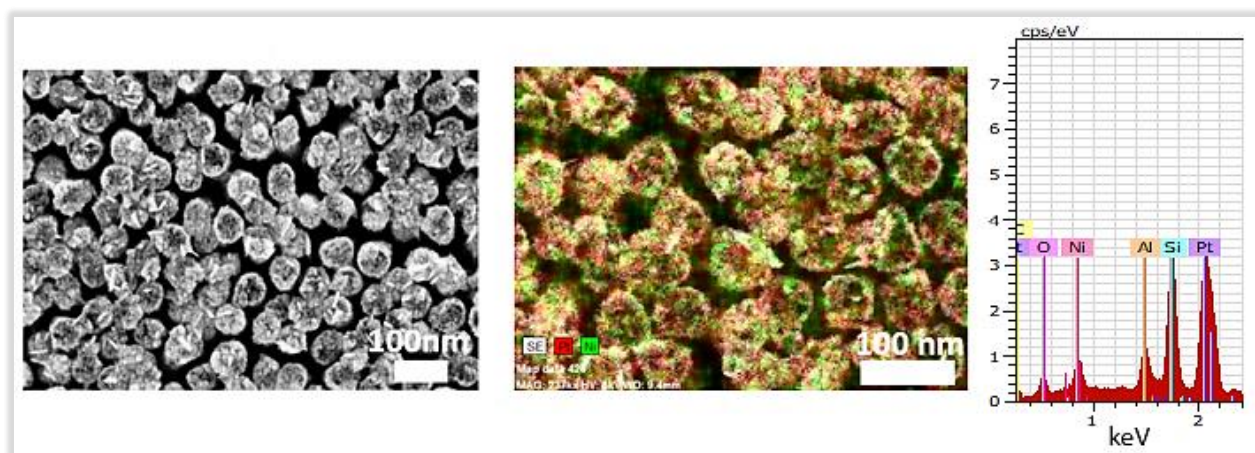
Figure III-80: SEM top-view structural characterization coupled with EDX elemental mapping of PtNiNWs after exposing NiNWs to a K_2PtCl_4 solution in 0.05 M HCl at 35°C for 8 minutes.
