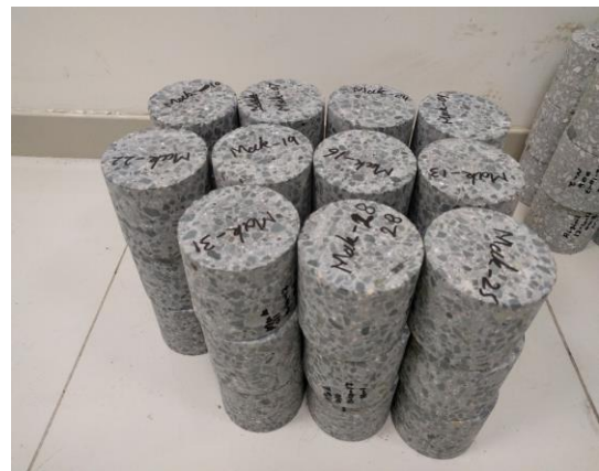
Figure 2.2 - Cores Drilled for Chloride Diffusion Test
