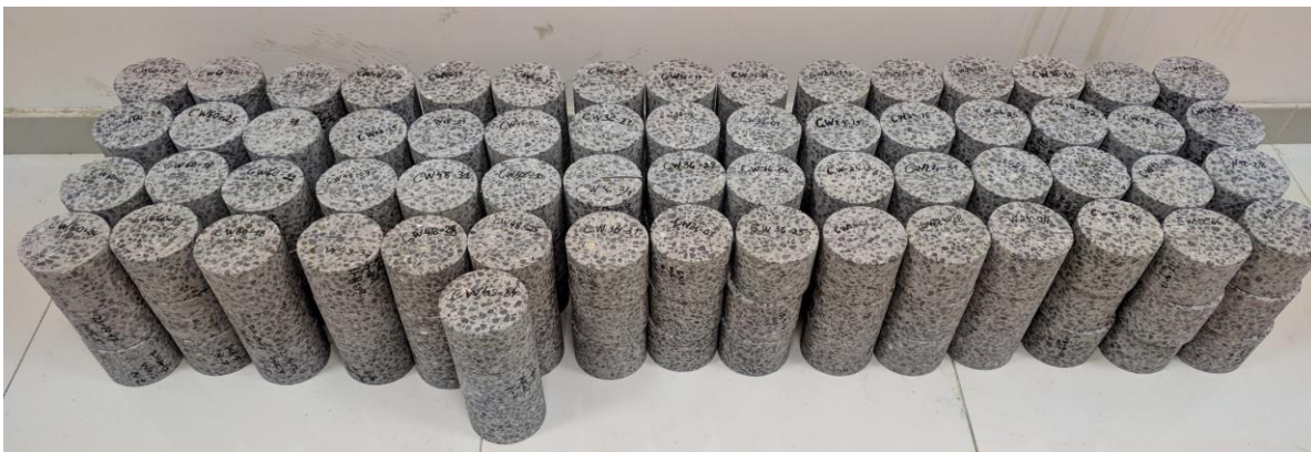
Figure 5.7 - Cores Drilled for Chloride Diffusion Test
