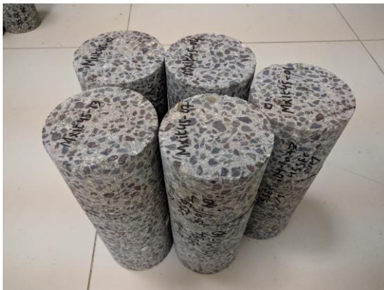
Figure 4.13 - Cores Drilled for Chloride Diffusion Test - MIXT Series
