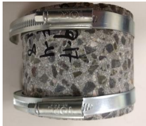
Figure 5.5 - Concrete Core Jointed by Steel Rings
