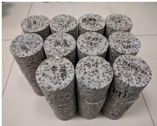
Figure 2.2 - Cores Drilled for Chloride Diffusion Test
