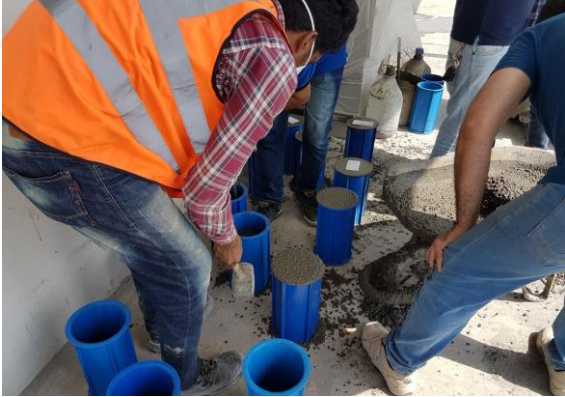
Figure 4.10 - Concrete Cylinders Preparation
