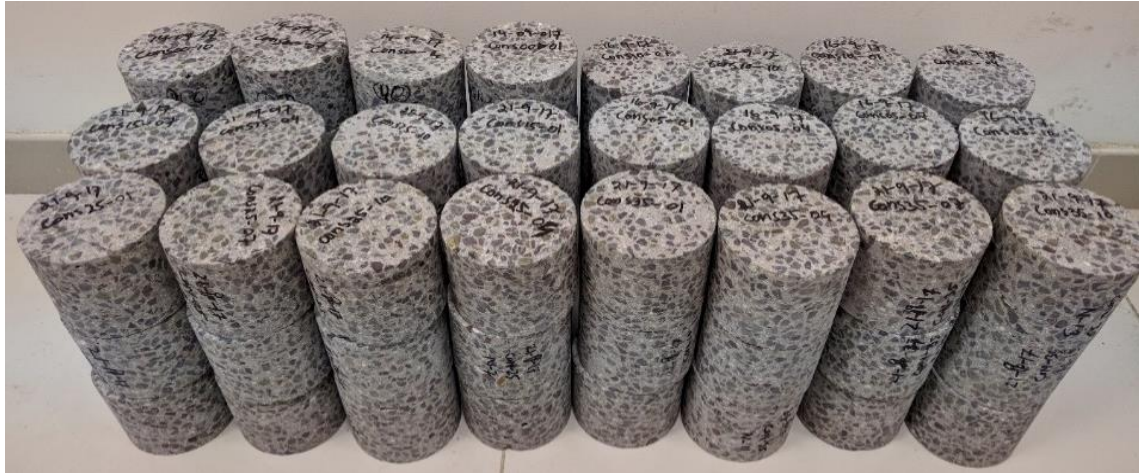
Figure 4.14 - Cores Drilled for Chloride Diffusion Test – CONS Series
