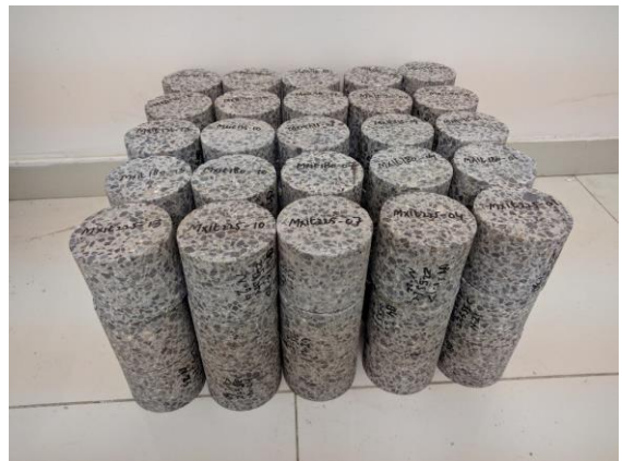
Figure 4.13 - Cores Drilled for Chloride Diffusion Test - MIXT Series
