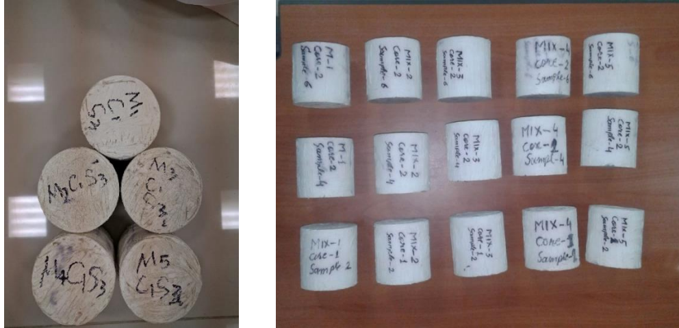
Figure 3.5 - Specimens Before Immersion in NaCl Solution
