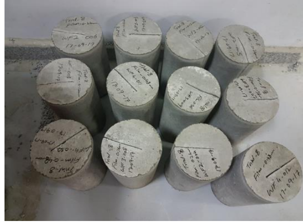
Figure 5.3 - Method 2 of Cracks Formation - Plastic Sheet Inserts
