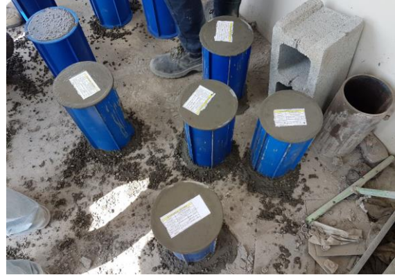
Figure 4.11 - Concrete Cylinders Preparation
