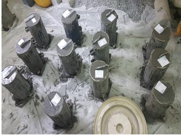
Figure 5.3 - Method 2 of Cracks Formation - Plastic Sheet Inserts
