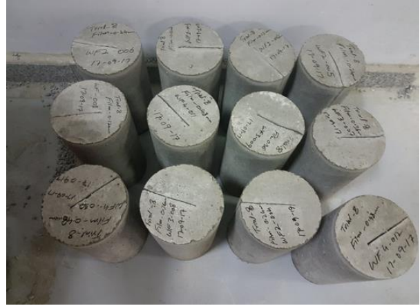
Figure 5.3 - Method 2 of Cracks Formation - Plastic Sheet Inserts
