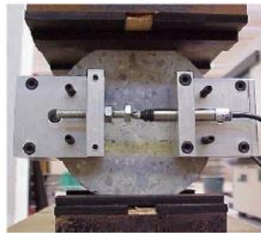
Fig. 1. Controlled splitting test.
