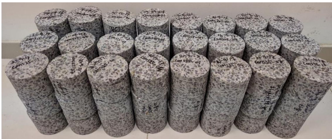
Figure 4.14 - Cores Drilled for Chloride Diffusion Test – CONS Series
