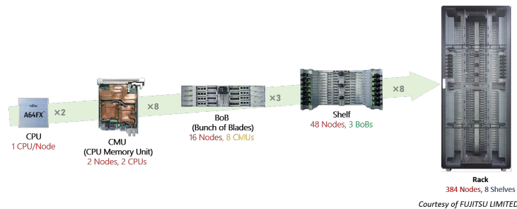
Figure 2.4: Hierarchy of Fugaku processing units [28].
