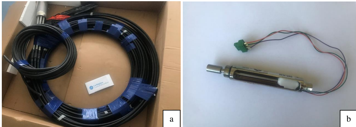
Figure 2.19 (a) Fiberglass rod extensometer and (b) one of its potentiometers
