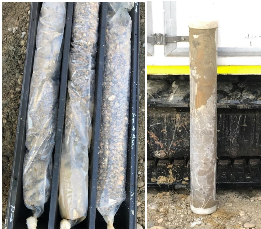
Figure 4.2 Disturbed and undisturbed samples extracted from the sonic drill
