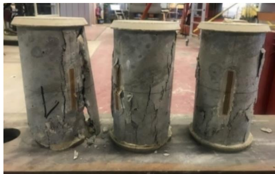
Figure 2.6 The three concrete cylindrical samples after the first batch of crushing tests
