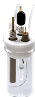
Figure PE-81 VC-4 cell with, from left to right glassy carbon electrode (WE), silver non-aqueous reference electrode (RE) and platinum wire (CE)
