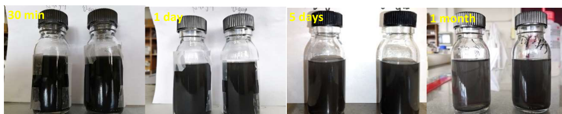
Fig. 2.3. Stability of NFG (left) and OFG (right) in the solvent: 0.22 g GNPs in 20 g solvent.
