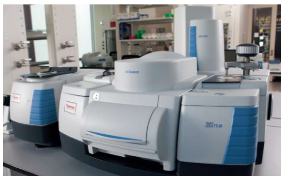
Fig. 2.9. Nicolet IS50R Thermo Fisher infrared spectroscopy for FTIR measurement.
