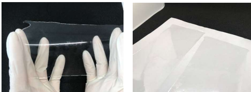
Fig. 2.5. The obtained polyurethane films with a thickness of about 100 \mu\text{m} .
