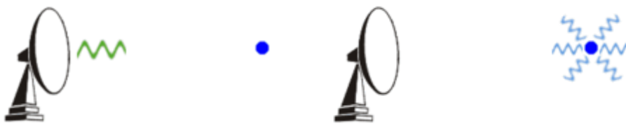
Figure 2-2 Illustration of an incident waves (a) transmitted by a source on the left that is scattered in all the directions by an obstacle on the right (b) [27].
