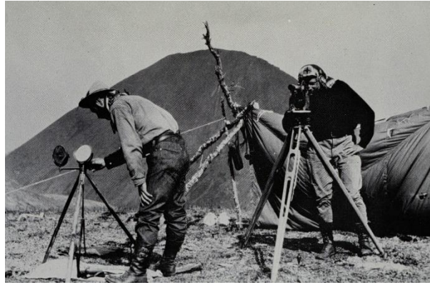
Figure 2-1 Heliograph, on the left, composed of a pivoting mirror allowing the transmission of data in Morse code. On the right an operator decoding the message from another heliograph [25].
