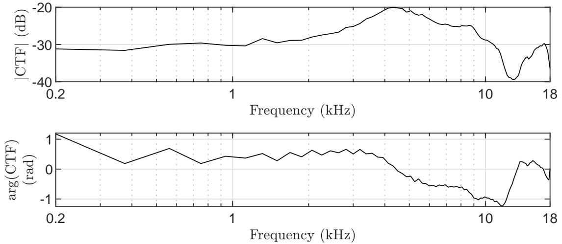
Figure 1.7 – Exemplary CTF, computed from the HRTF set of subject NH8 of the ARI dataset using the RMS averaging method.
