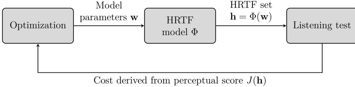
Figure 4.1 – General architecture of the HRTF tuning method.
