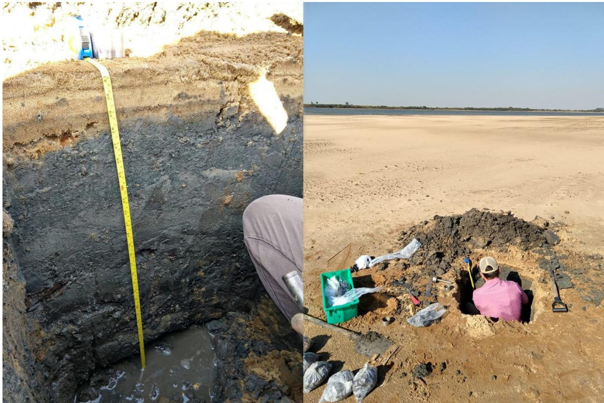
Figure 5.7. Sediment sampling in a deposit within an island of the Uruguay River. Source: the author.
