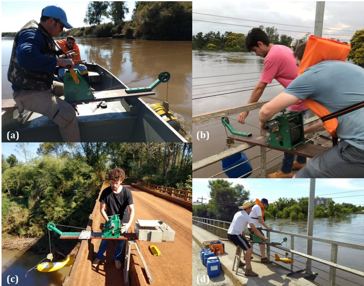
Figure 5.5. Suspended sediment sampling to determine the concentration during a monitoring campaign made in collaboration with the National Water Agency service provider, the Brazilian Geological Service (CPRM) (a); Event sampling in the Ibirapuitã River during a storm event, sample taken with a bucket to obtain larger volumes (b) and for suspended sediment concentration collected with a US-D49 sampler (d); Suspended sediment sampling in the Conceição River before a storm event using a US-D49 on a bridge (c). Source: the author (a, c), Paulo C. Ramon (b), Antônio A. Marquez (d).
