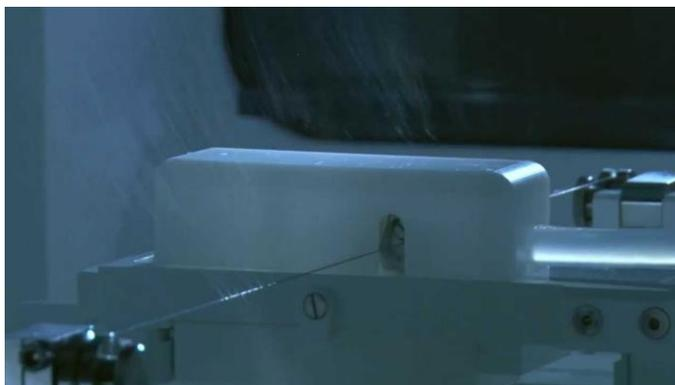
**Figure 4.1. Nanofibers production from a polymer solution coated wire electrode and a solution carriage moving across its length**
