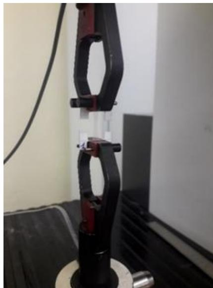
**Figure 2.5. Specimen between the jaws of MTS M/20 Tester**
