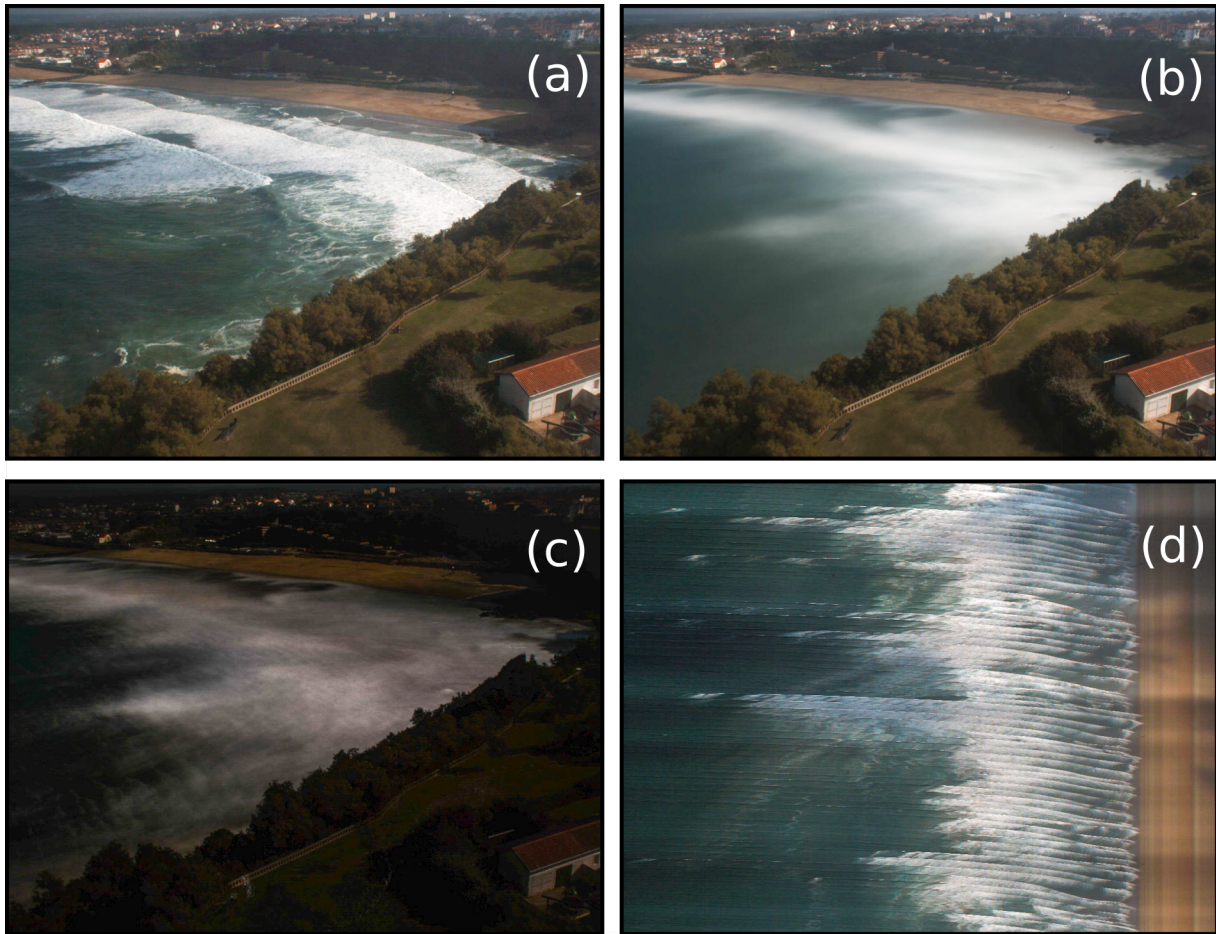
Figure 1.2 – Typical standard video-derived products. (a) Snapshot, (b) timex, (c) variance and (d) timestack image.
