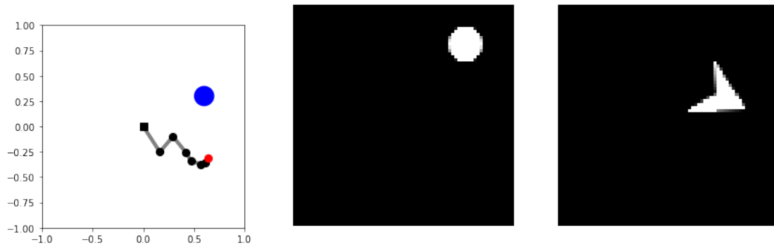
Figure 1: Left: The Arm-Ball environment with a 7 DOF arm, controlled by a 21D continuous actions DMP controller, that can stick and move the ball if the arm tip touches it (on the left). Right: rendered 70x70 images used as raw signals representing the end position of the objects for Arm-Ball (on the center) and Arm-Arrow (on the right) environments. The arm is not visible to learners.
