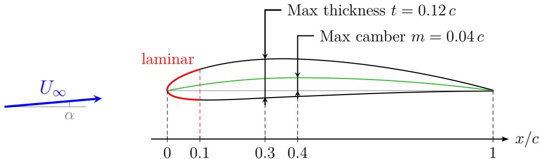
**Figure 5.2:** The NACA 4412 wing profile geometry
