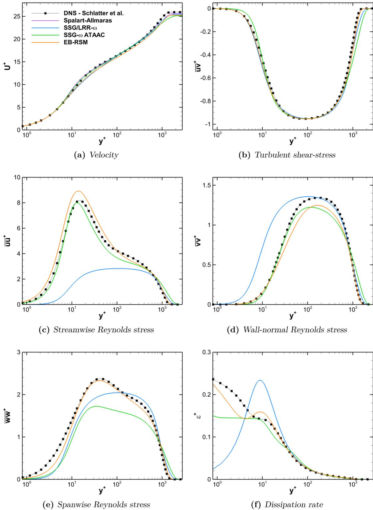
Figure 4.5: Profiles on the flat plate at  $Re_\theta = 4,060$
