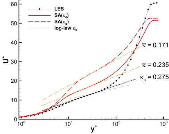
Figure 2: SA( $\kappa_0$ ) and SA( $\kappa_p$ ) models velocity profiles on the NACA 4412 wing section at  $p^+ = 0.151$
