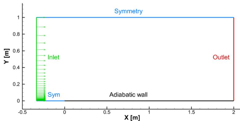
Figure 4.1: Computational domain of the flat plate
