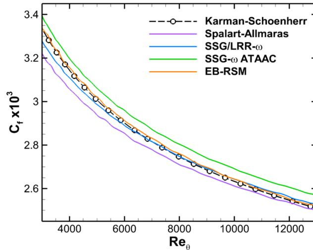
**Figure 4.4:** Skin friction coefficient on the flat plate
