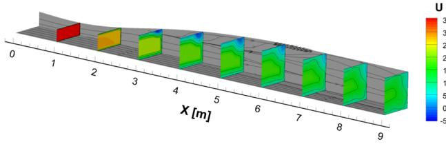
Figure 9: Flow topology for the Spalart-Allmaras QCR model. The lines indicate the skin friction direction.
