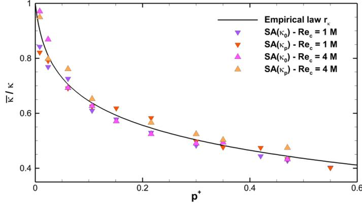
**Figure 5.5:** Apparent-to-target  $\kappa$  ratio for the Spalart-Allmaras model
