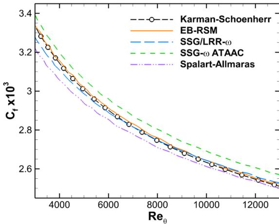
Figure 2: Skin friction coefficient on the flat plate
