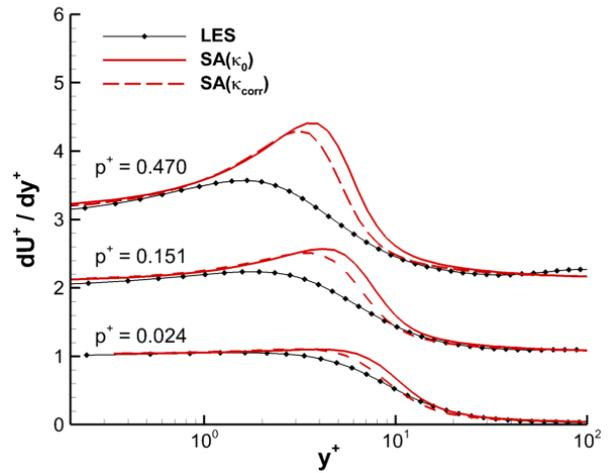
Figure 11: SA( $\kappa_0$ ) and SA( $\kappa_{corr}$ ) models  $dU^+/dy^+$  profiles in the viscous sublayer on the NACA 4412 wing section for three pressure gradients (the profiles are shifted incrementally)
