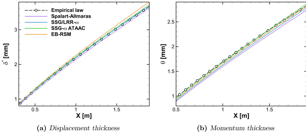
**Figure 4.3:** Boundary layer thicknesses on the flat plate
