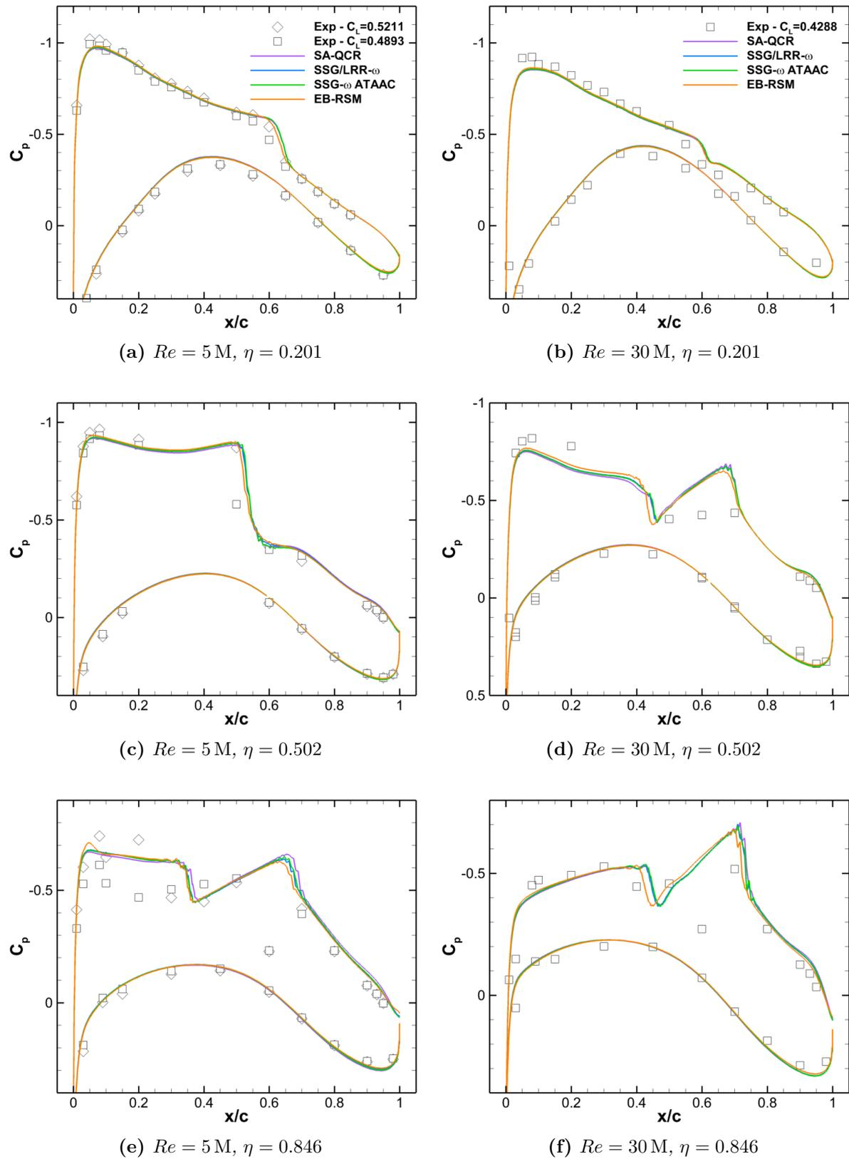
**Figure 7.3:** Pressure coefficients on the CRM
