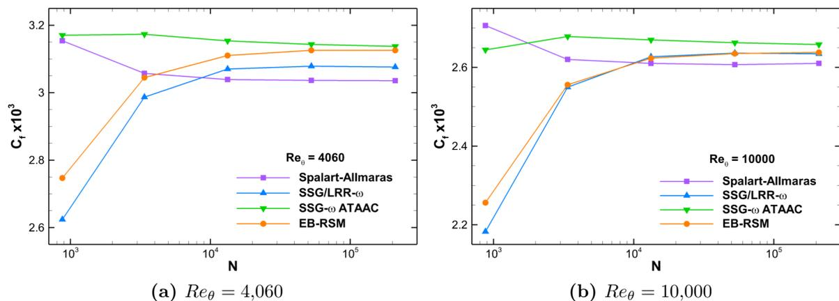
**Figure 4.2:** Mesh convergence for the flat plate
