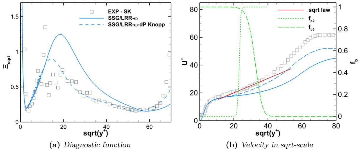
**Figure 6.4:** Square-root behaviour in the Skåre & Krogstad test case at  $x = 5.0$  m for the SSG/LRR- $\omega$  and the SSG/LRR- $\omega$ -dP Knopp models
