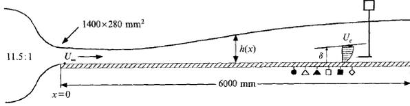
Figure 12: Skåre & Krogstad experiment configuration [14]
