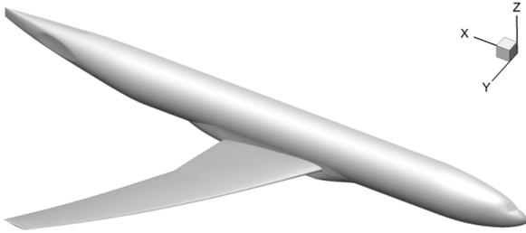
Figure 17: The CRM "Wing and Body" configuration
