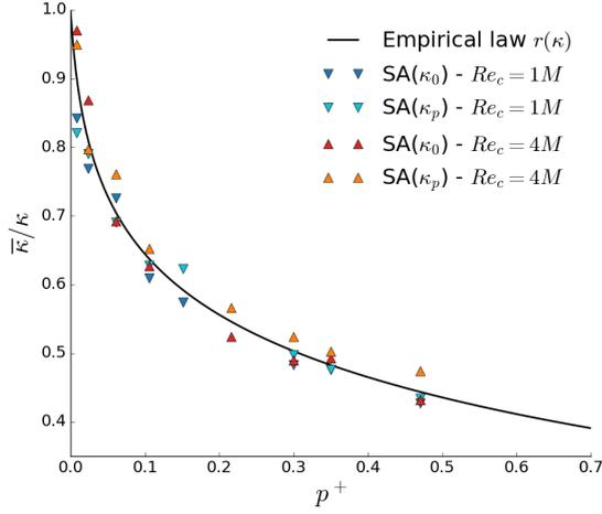
Figure 5: Apparent-to-target  $\kappa$  ratio for the Spalart-Allmaras model
