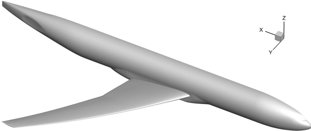
**Figure 7.1:** *The CRM ‘Wing-Body’ configuration*
