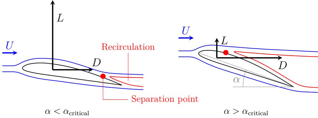
**Figure 2.1:** Lift and drag on a wing profile
